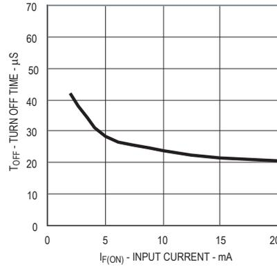
Figure 11. Typical Turn Off Time vs. Input Current
