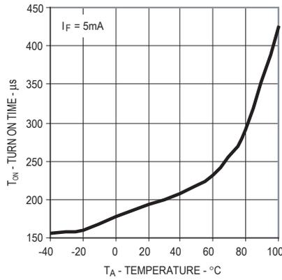
Figure 10. Typical Turn On Time vs. Temperature
