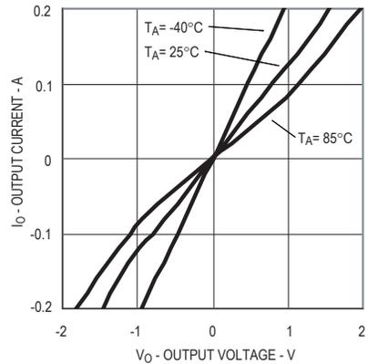
Figure 8. Typical Output Current vs. Output Voltage
