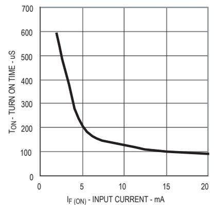
Figure 9. Typical Turn On Time vs. Input Current
