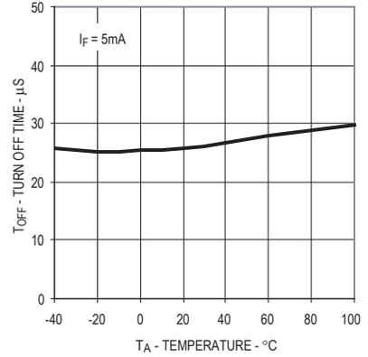
Figure 12. Typical Turn Off Time vs. Temperature
