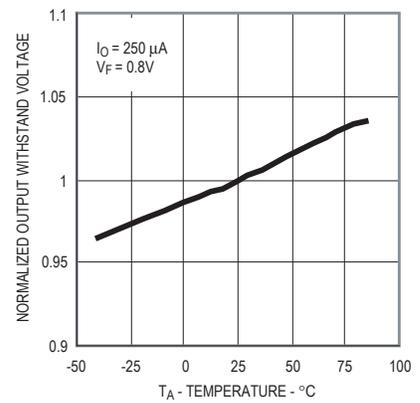
Figure 3. Normalized Typical Output Withstand Voltage vs. Temperature
