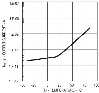
Figure 4. Typical Output Leakage Current vs. Temperature
