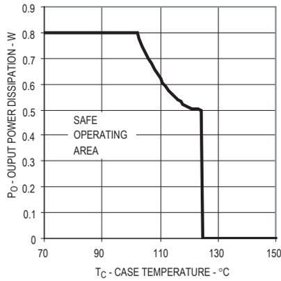
Figure 2. Output Power Derating vs Case Temperature
