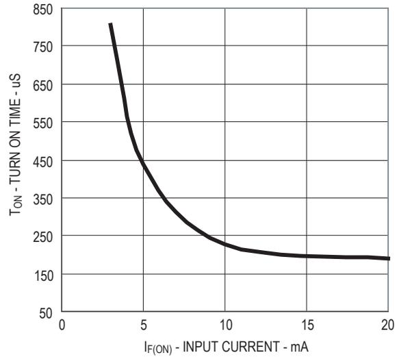
Figure 12. Typical Turn On Time vs. Input Current
