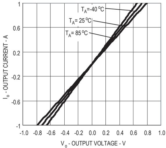
Figure 11. Typical Output Current vs. Output Voltage
