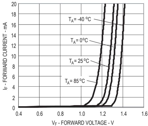
Figure 9. Typical Forward Current vs. Forward Voltage
