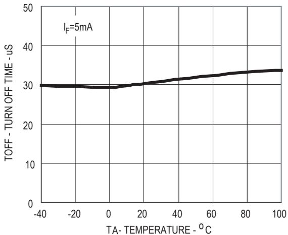
Figure 15. Typical Turn Off Time vs. Temperature
