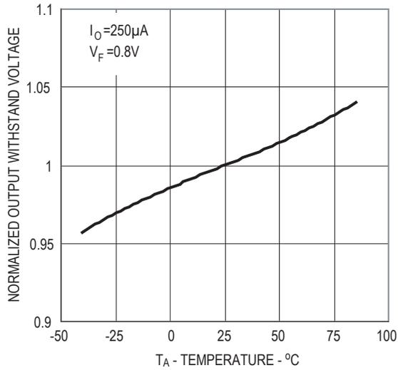
Figure 5. Normalized Typical Output Withstand Voltage vs. Temperature
