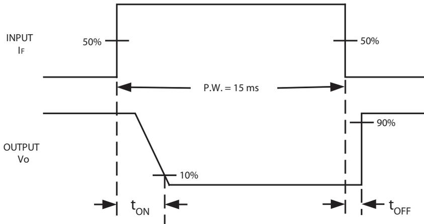
Figure 16. Switching Test circuit for  $t_{ON}$ ,  $t_{OFF}$
