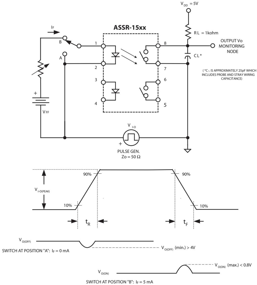
**Figure 18. Input - Output Transient Rejection Test Circuit**
