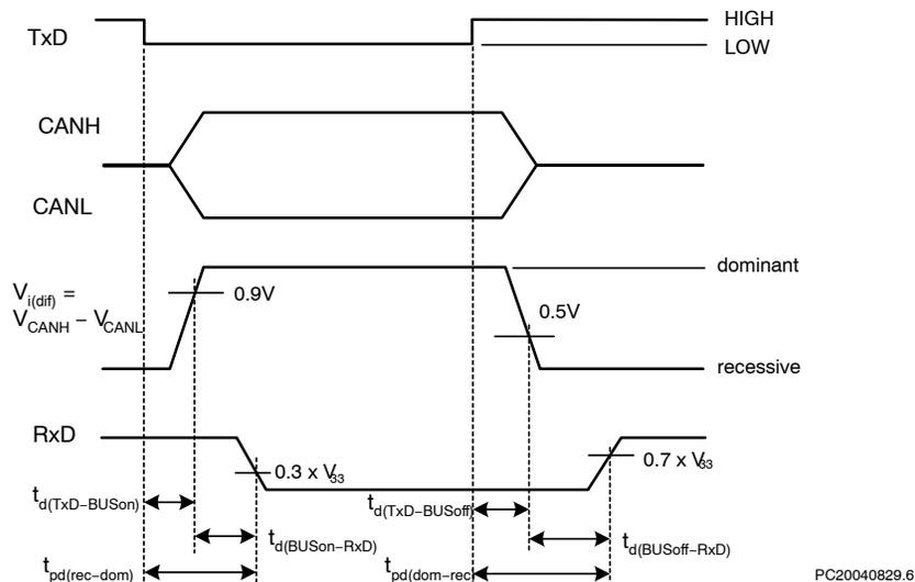
Figure 6. Timing Diagram for AC Characteristics
