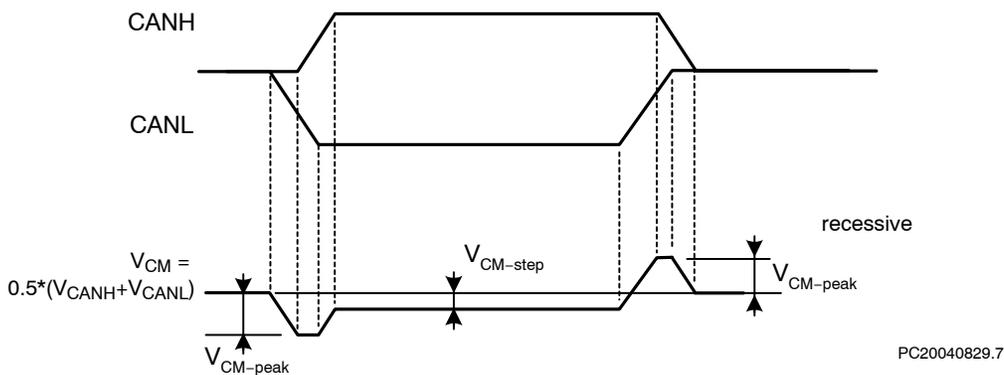
Figure 8. Common-Mode Voltage Peaks (See Measurement Setup Figure 7)
