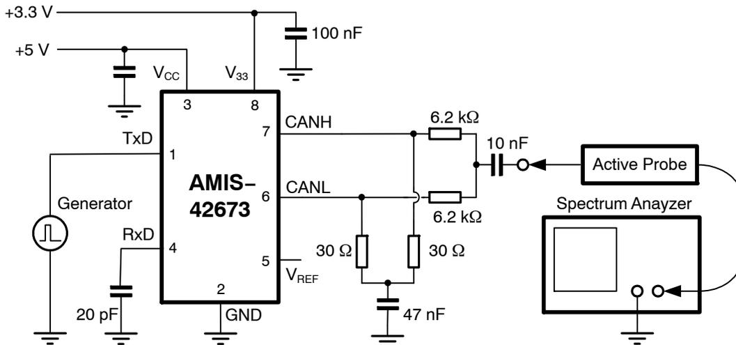
Figure 7. Basic Test Setup for Electromagnetic Measurement
