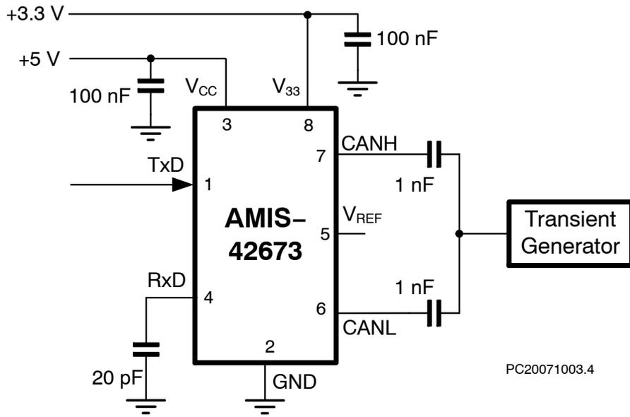
Figure 3. Test Circuit for Automotive Transients
