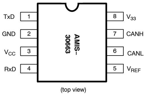
Figure 3. Pin Configuration
