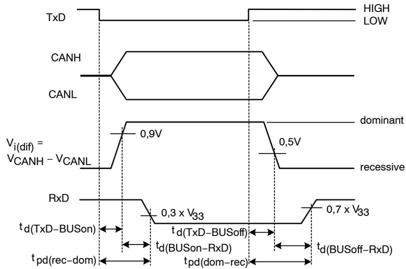
Figure 7. Timing Diagram for AC Characteristics
