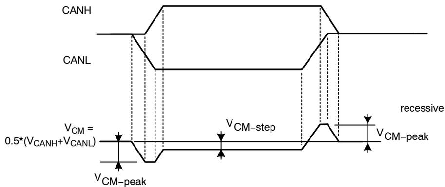
Figure 9. Common-mode Voltage Peaks (see measurement set-up Figure 8)
