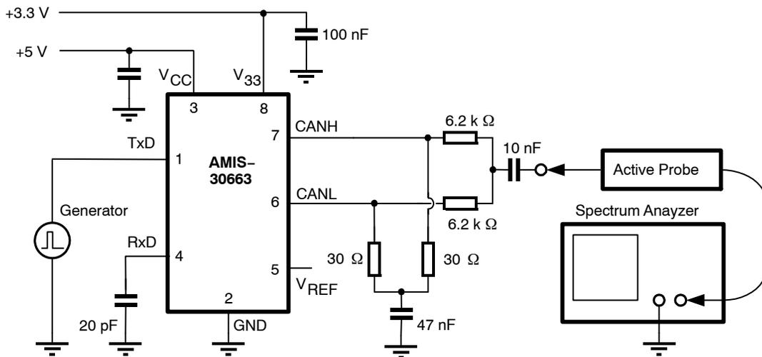
Figure 8. Basic Test Set-up for Electromagnetic Measurement
