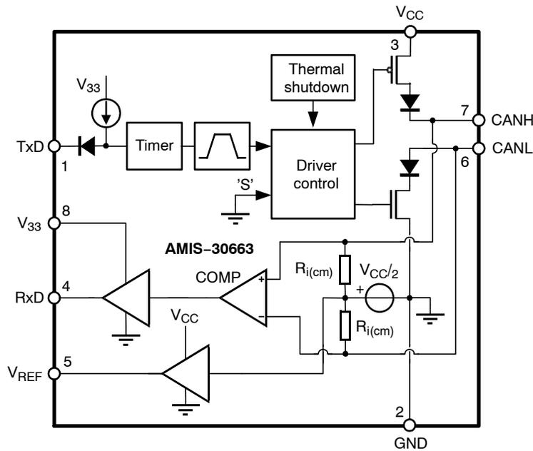
Figure 1. Block Diagram
