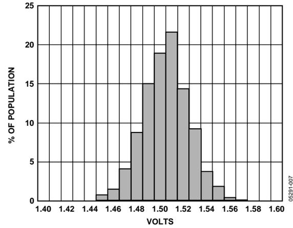
Figure 7. Y-Axis Zero g Bias at 25°C
