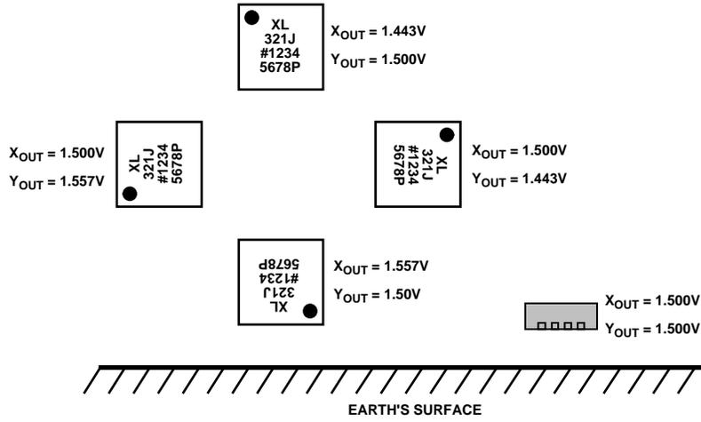
Figure 20. Output Response vs. Orientation (Top View)
