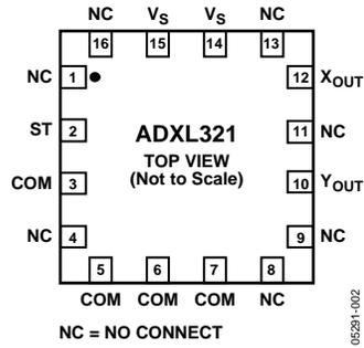
Figure 2. Pin Configuration
