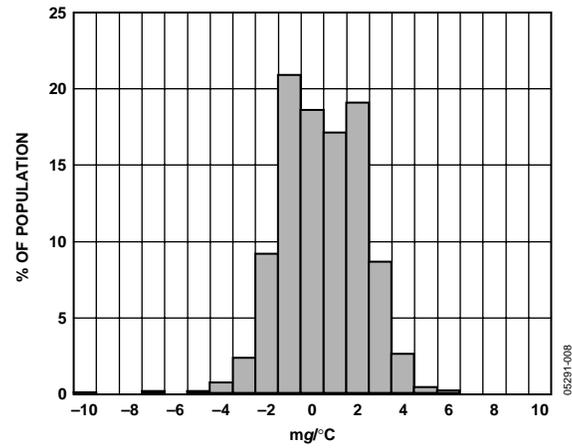
Figure 8. Y-Axis Zero g Bias Temperature Coefficient
