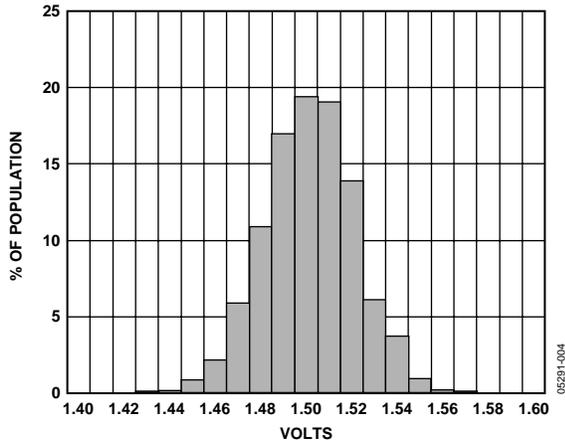
Figure 4. X-Axis Zero g Bias at 25°C
