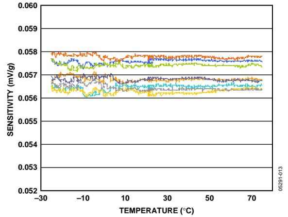
Figure 13. Sensitivity vs. Temperature—Parts Soldered to PCB
