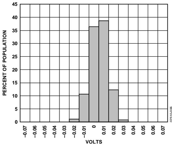
Figure 6. Zero-g Bias Deviation from Ideal ( $T_A = 125^\circ\text{C}$ )
