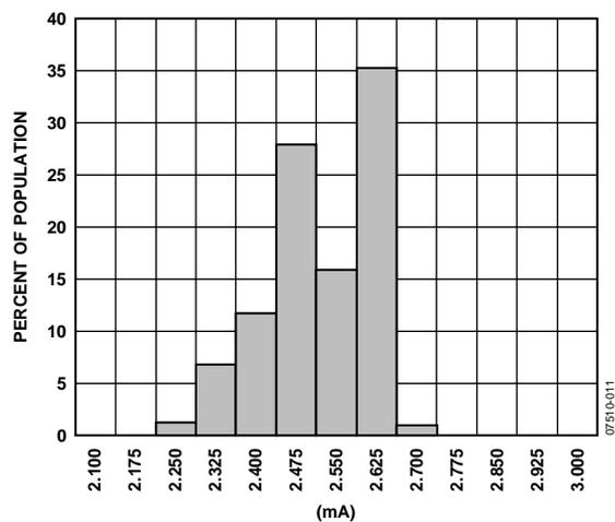
Figure 11.  $I_{SUPPLY}$  at 125°C
