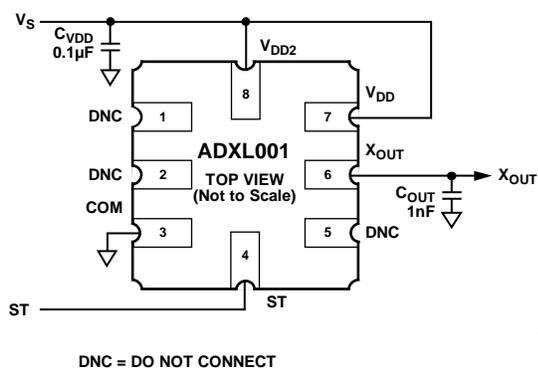
Figure 14. Application Circuit
