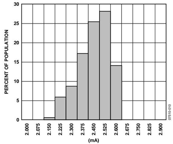
Figure 10.  $I_{SUPPLY}$  at  $25^\circ\text{C}$
