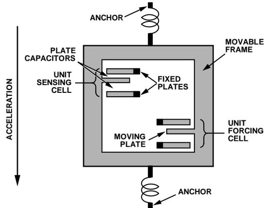
Figure 13. Simplified View of Sensor Under Acceleration
