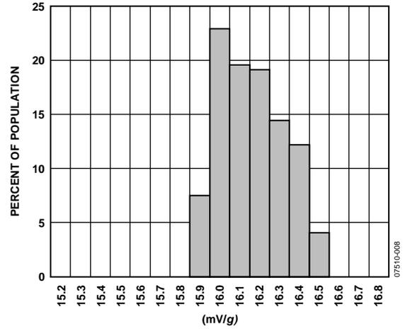
Figure 8. Sensitivity Distribution ( $T_A = 125^\circ\text{C}$ )
