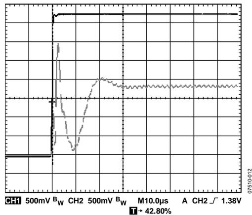
Figure 12. Turn-On Characteristic (10 μs per DIV)
