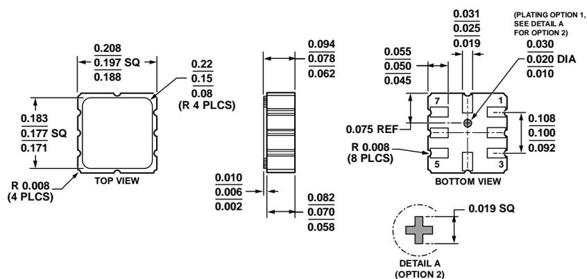
Figure 17. 8-Terminal Ceramic Leadless Chip Carrier [LCC]
