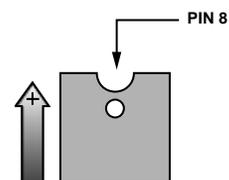
Figure 15.  $X_{OUT}$  Increases with Acceleration in the Positive X-Axis Direction
