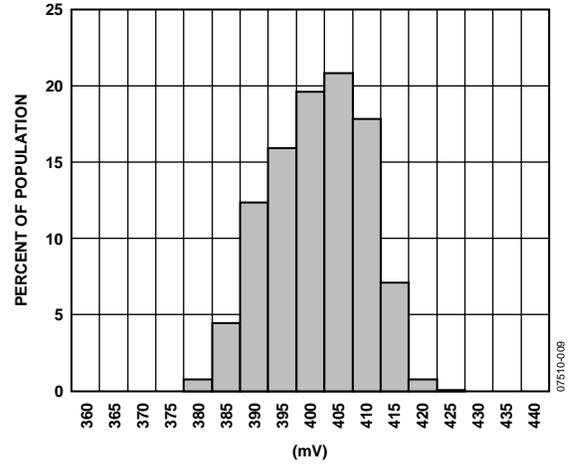
Figure 9. Self-Test Delta
