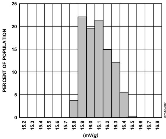
Figure 7. Sensitivity Distribution (3.3 V Supply,  $25^\circ\text{C}$ )
