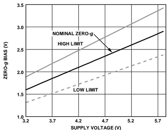
Figure 16. Typical Zero-g Bias Levels Across Varying Supply Voltages
