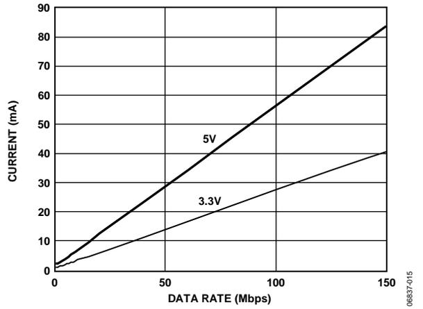
Figure 15. Typical ADuM3442 V<sub>DD1</sub> or V<sub>DD2</sub> Supply Current vs. Data Rate for 5 V and 3.3 V Operation
