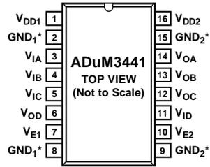
\*PIN 2 AND PIN 8 ARE INTERNALLY CONNECTED AND CONNECTING BOTH TO GND<sub>1</sub> IS RECOMMENDED. PIN 9 AND PIN 15 ARE INTERNALLY CONNECTED AND CONNECTING BOTH TO GND<sub>2</sub> IS RECOMMENDED.
