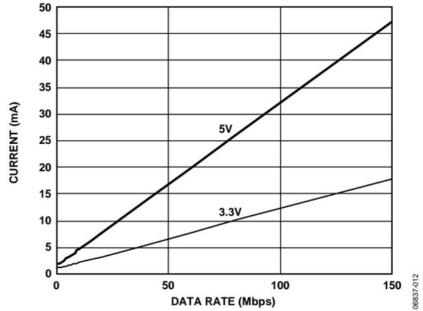
Figure 12. Typical ADuM3440 V<sub>DD2</sub> Supply Current vs. Data Rate for 5 V and 3.3 V Operation
