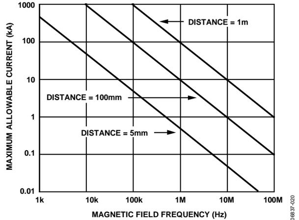
Figure 19. Maximum Allowable Current for Various Current-to-ADuM344x Spacings
