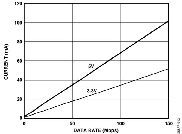
Figure 13. Typical ADuM3441 V<sub>DD1</sub> Supply Current vs. Data Rate for 5 V and 3.3 V Operation
