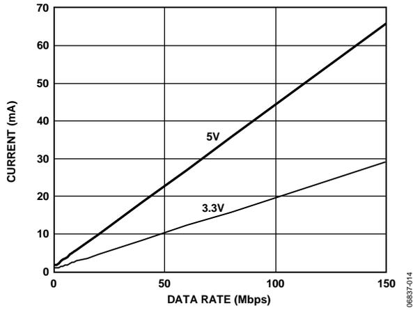
Figure 14. Typical ADuM3441 V<sub>DD2</sub> Supply Current vs. Data Rate for 5 V and 3.3 V Operation
