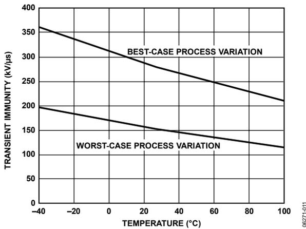
Figure 8. Transient Immunity (Linear Transients) vs. Temperature
