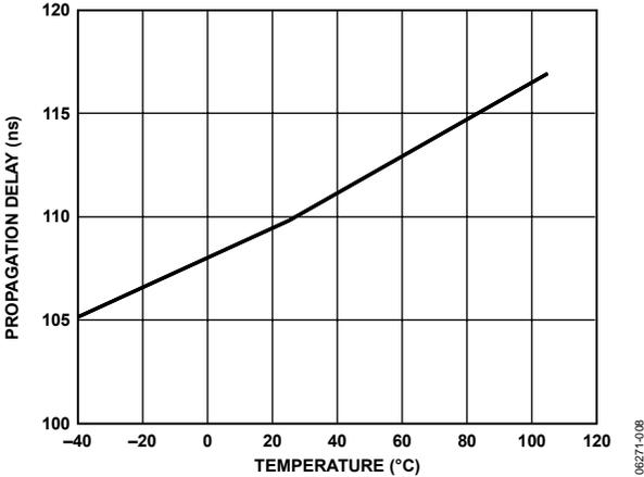
Figure 5. Typical Propagation Delay Variation with Temperature
