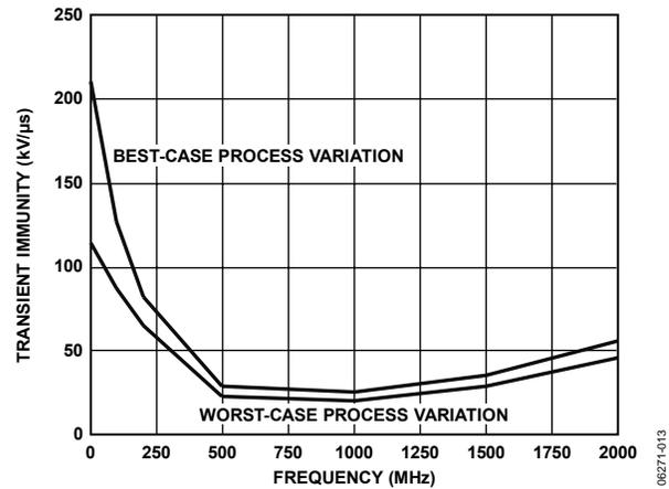
Figure 10. Transient Immunity (Sinusoidal Transients), 100°C Ambient Temperature
