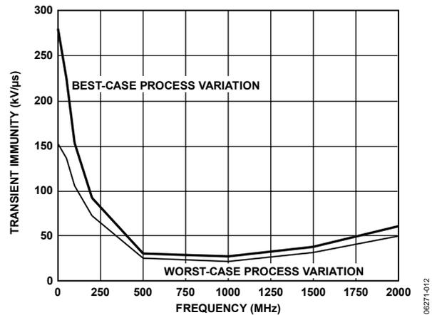
Figure 9. Transient Immunity (Sinusoidal Transients), 27°C Ambient Temperature
