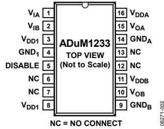
Figure 2. Pin Configuration
