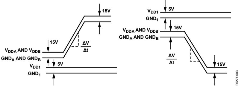
Figure 11. Common-Mode Transient Immunity Waveforms—Input to Output
