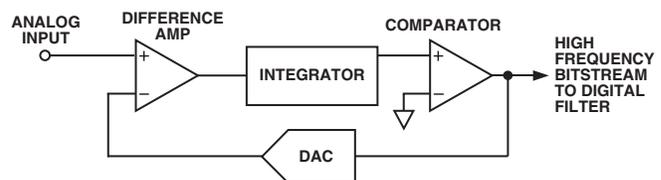
Figure 10.  $\Sigma$ - $\Delta$  Modulator Simplified Block Diagram
