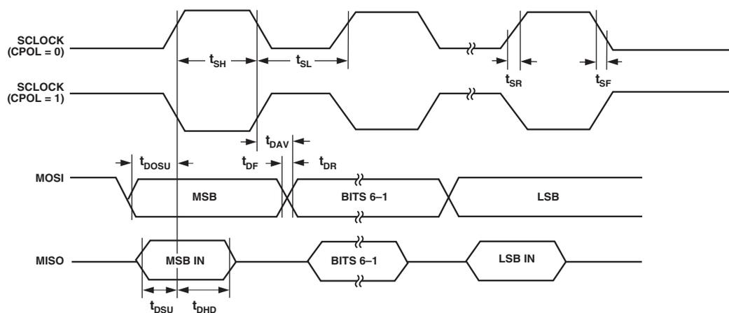
Figure 75. SPI Master Mode Timing (CPHA = 1)
