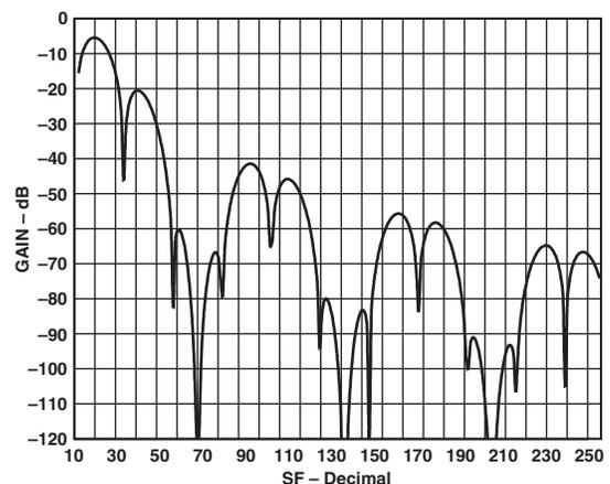
Figure 14. 60 Hz Normal Mode Rejection vs. SF
