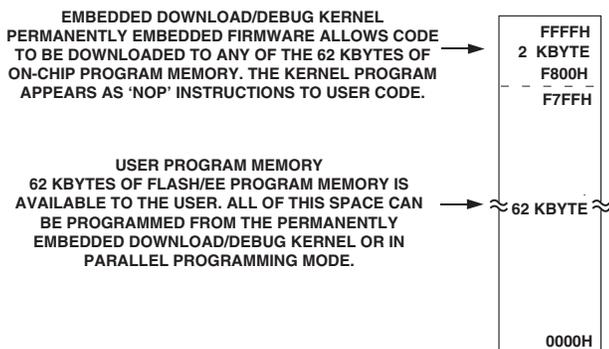
Figure 17. Flash/EE Program Memory Map in Normal Mode
