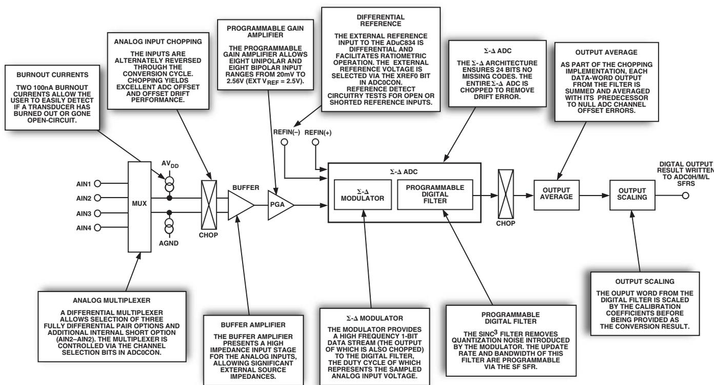
Figure 7. Primary ADC Block Diagram
