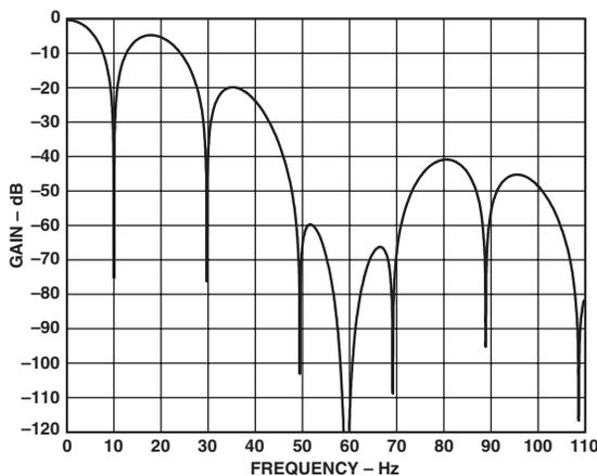
Figure 11. Filter Response, SF = 69 dec
