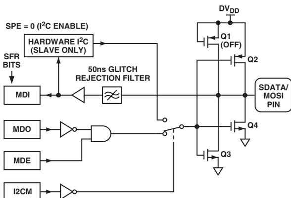
Figure 45. SDATA/MOSI Pin I/O Functional Equivalent in I<sup>2</sup>C Mode
