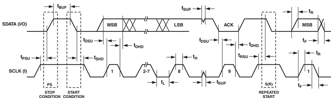
Figure 79. I<sup>2</sup>C Compatible Interface Timing
