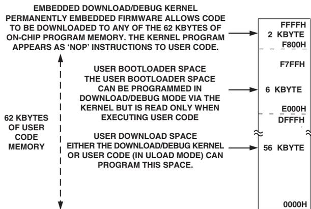
Figure 19. Flash/EE Program Memory Map in ULOAD Mode
