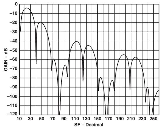
Figure 13. 50 Hz Normal Mode Rejection vs. SF
