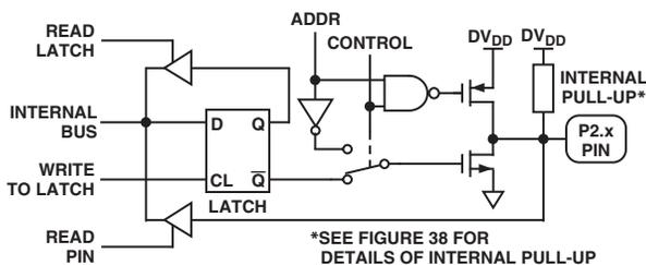
Figure 40. Port 2 Bit Latch and I/O Buffer
