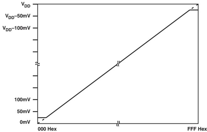
Figure 22. Endpoint Nonlinearities Due to Amplifier Saturation
