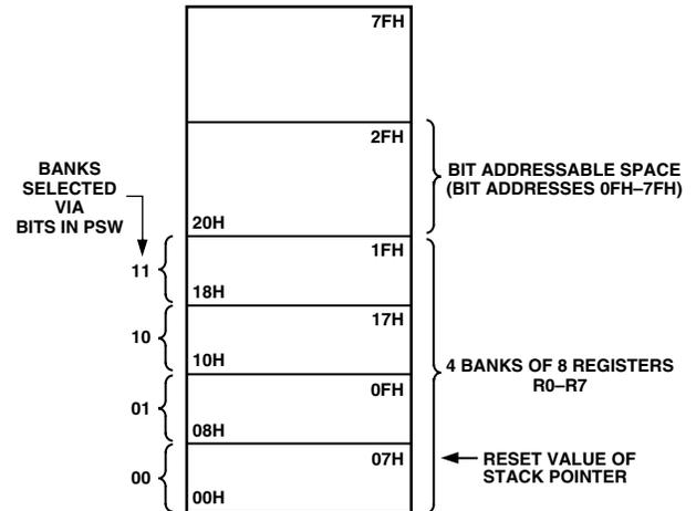
Figure 2. Lower 128 Bytes of Internal RAM
