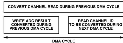
Figure 13. DMA Cycle
