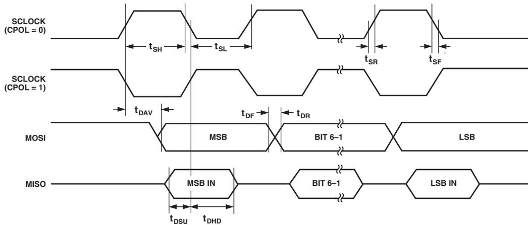
Figure 56. SPI Master Mode Timing (CPHA = 1)
