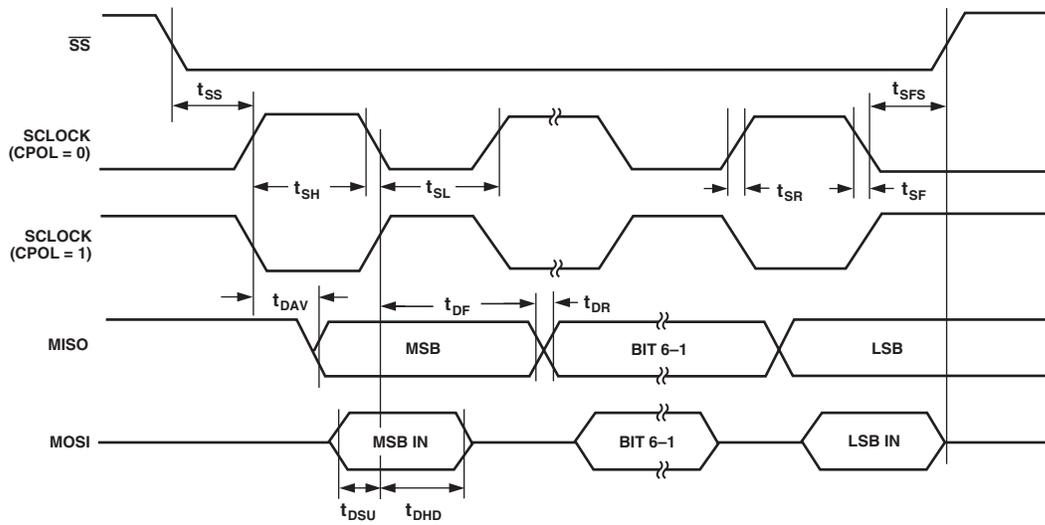
Figure 58. SPI Slave Mode Timing (CPHA = 1)
