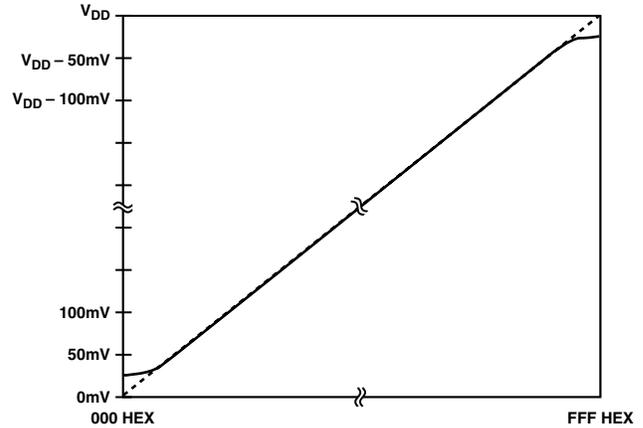
Figure 19. Endpoint Nonlinearities Due to Amplifier Saturation
