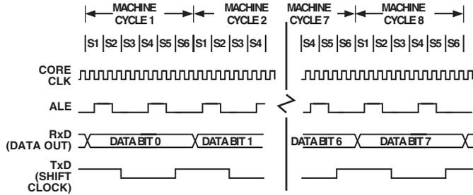
Figure 32. UART Serial Port Transmission, Mode 0
