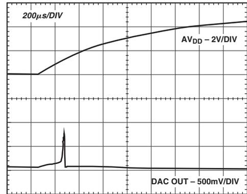
Figure 23. DAC Output Spike at Chip Power-Up
