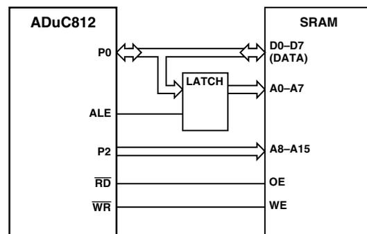
Figure 38. External Data Memory Interface (64K Address Space)
