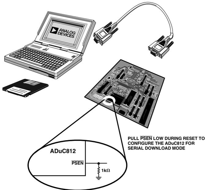
Figure 15. Flash/EE Memory Serial Download Mode Programming
