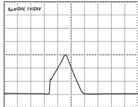
Figure 24. DAC Output Spike at DAC Enable
