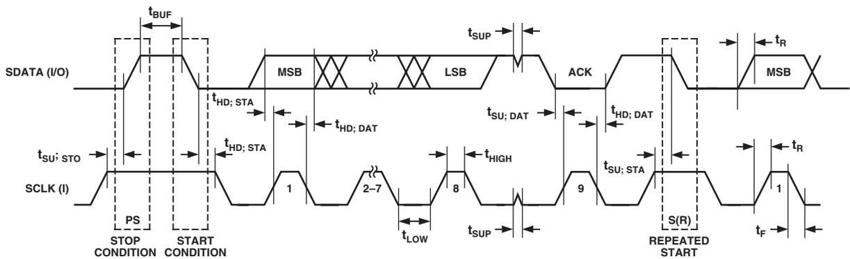
Figure 55. I<sup>2</sup>C Compatible Interface Timing
