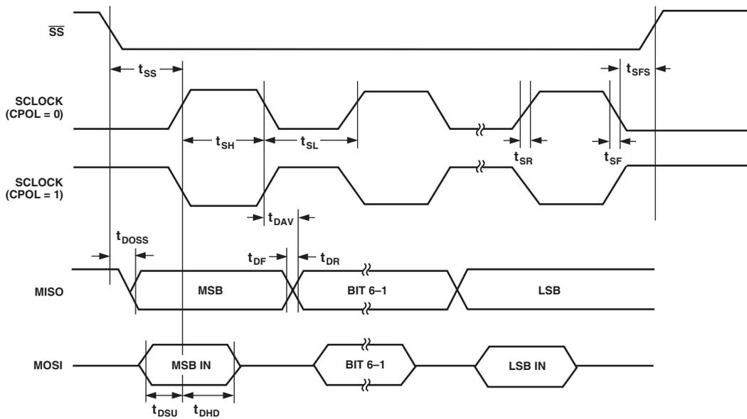
Figure 59. SPI Slave Mode Timing (CPHA = 0)
