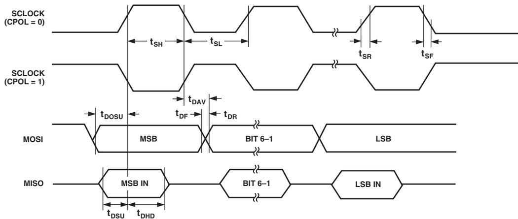
Figure 57. SPI Master Mode Timing (CPHA = 0)
