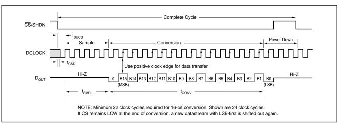
FIGURE 3. ADS8320 Basic Timing Diagrams.
