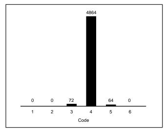
FIGURE 2. Histogram of 5000 Conversions of a DC Input at the Code Center.
