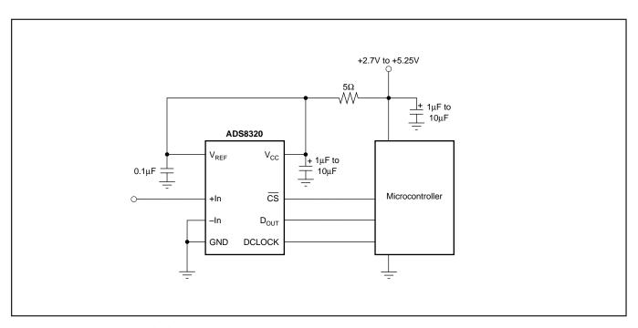
FIGURE 8. Basic Data Acquisition System.
