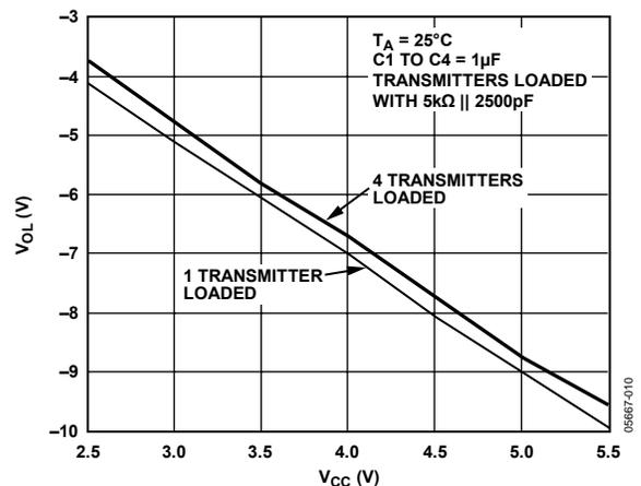
Figure 9. Transmitter Output Voltage Low vs.  $V_{CC}$
