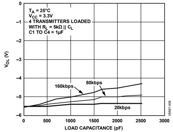
Figure 7. Transmitter Output Voltage Low vs. Load Capacitance
