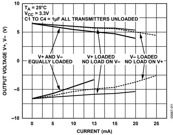
Figure 10.  $V_+$ ,  $V_-$  vs. Load Current
