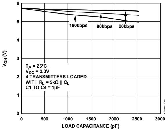
Figure 4. Transmitter Output Voltage High vs. Load Capacitance
