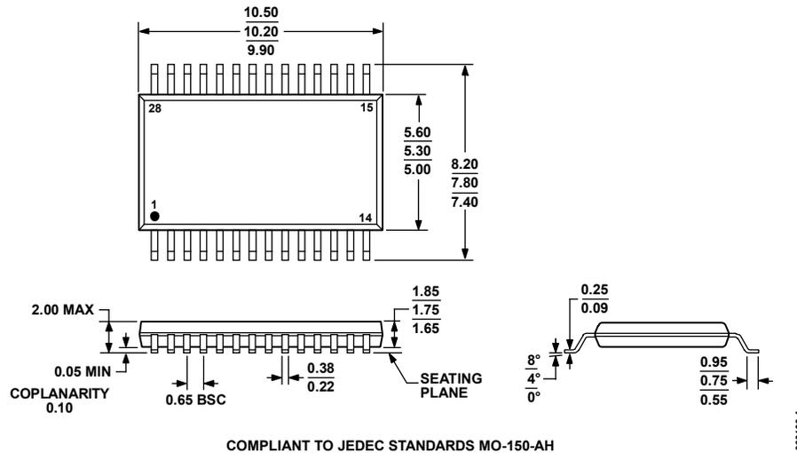
Figure 13. 28-Lead Shrink Small Outline Package [SSOP] (RS-28)
