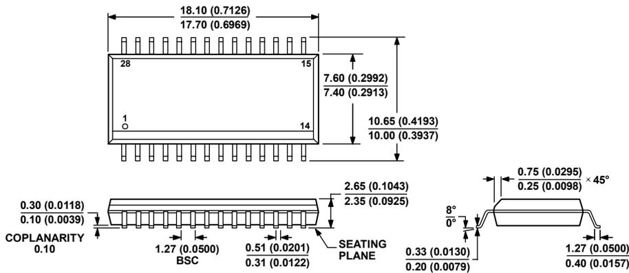
Figure 14. 28-Lead Standard Small Outline Package [SOIC\_W] Wide Body (RW-28)
