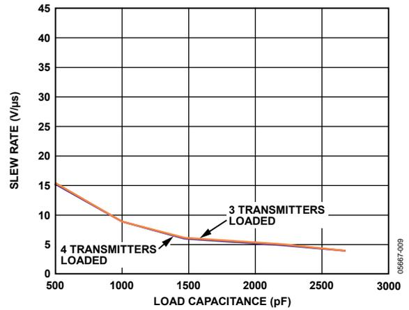
Figure 8. Transmitter Slew Rate vs. Load Capacitance
