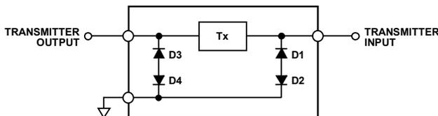
Figure 33. ADM3307E Transmitter Output Protection Scheme
