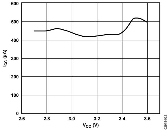
Figure 22. I<sub>CC</sub> vs. V<sub>CC</sub> (Unloaded)
