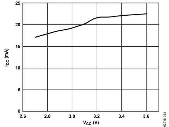
Figure 23. I<sub>CC</sub> vs. V<sub>CC</sub> (R<sub>L</sub> = 3 kΩ)
