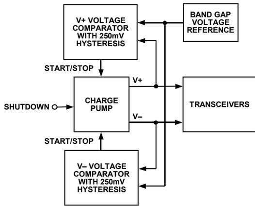
Figure 26. Block Diagram of Green Idle Circuit
