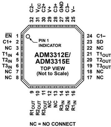
Figure 8. LFCSP\_VQ Pin Configuration
