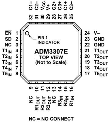
Figure 4. ADM3307E LFCSP\_VQ Pin Configuration
