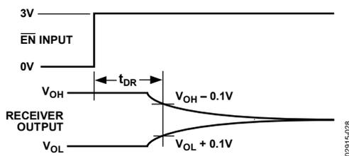
Figure 28. Receiver Disable Timing
