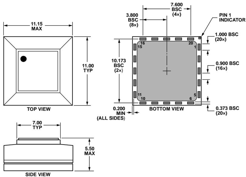
Figure 21. 20-Terminal Stacked Land Grid Array [LGA]
