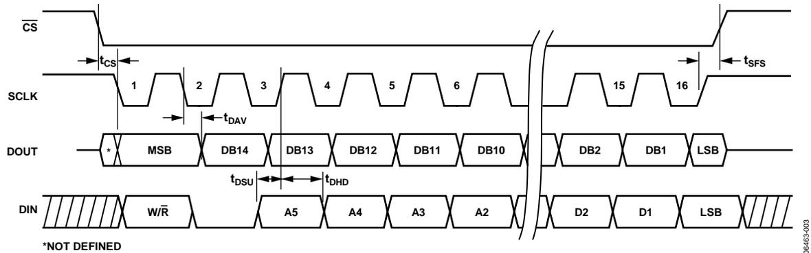
Figure 3. SPI Timing
