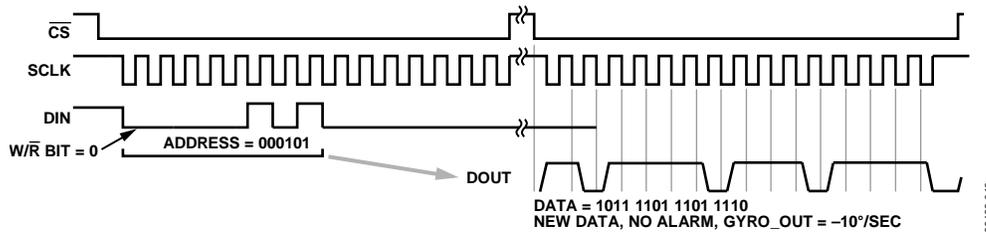
Figure 18. Example of a Read Cycle, ±80°/sec Setting
