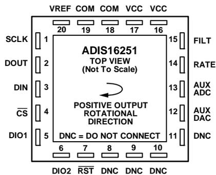
Figure 5. Pin Configuration
