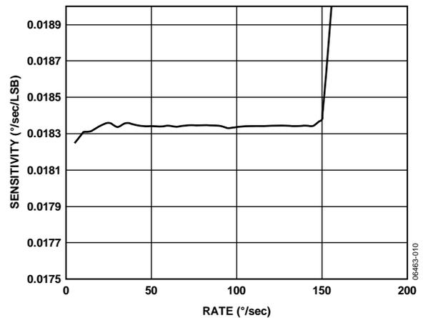
Figure 12. Sensitivity vs. Angular Rate,  $\pm 80^\circ/\text{sec}$  Range
