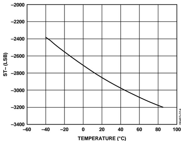
Figure 14. Negative Self-Test vs. Temperature
