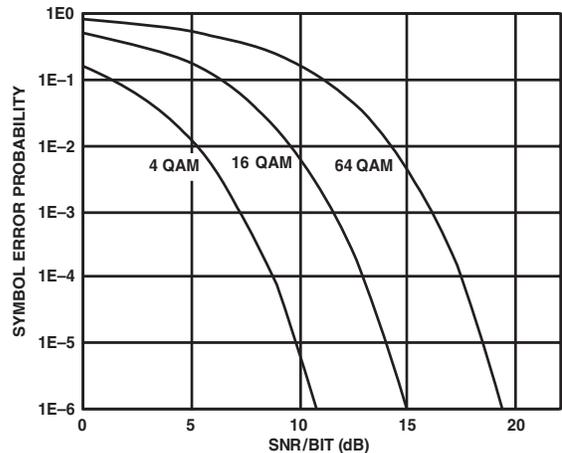
Figure 32. Probability of a Symbol Error for QAM
