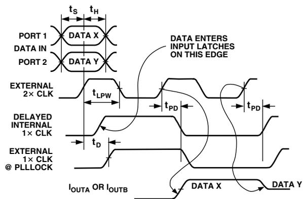
Figure 11. Timing Requirements, Interleaved (2×) Mode with PLL Disabled
