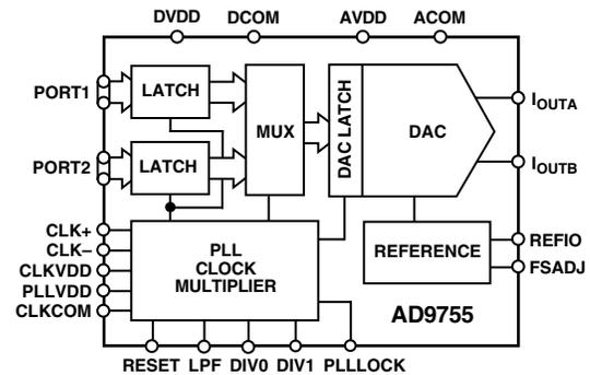
The DAC utilizes a segmented current source architecture combined with a proprietary switching technique to reduce glitch energy and maximize dynamic accuracy. Differential current outputs support single-ended or differential applications. The differential outputs each provide a nominal full-scale current from 2 mA to 20 mA.
