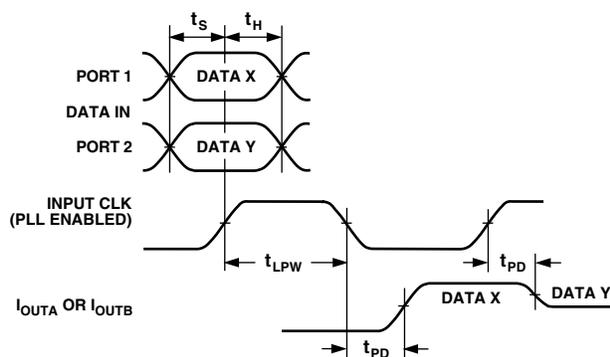
Figure 1. I/O Timing
