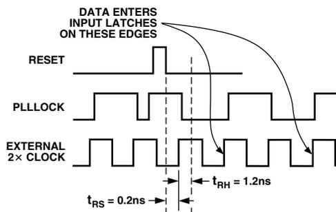
Figure 12. Reset Function Timing with PLL Disabled
