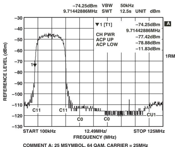
Figure 28. Reconstructed 64-QAM Signal at 25 MHz IF
