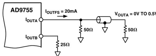
Figure 23. 0 V to 0.5 V Unbuffered Voltage Output
