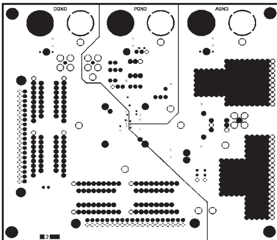
Figure 39. Evaluation Board, Layer 2, Ground Plane
