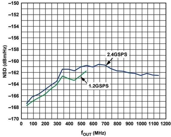
Figure 30. Single-Tone NSD vs.  $f_{OUT}$  over  $f_{DAC}$
