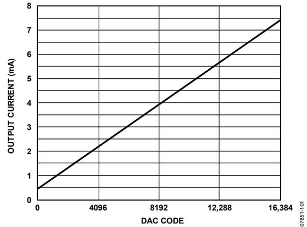
Figure 104. Gain Curve for FSC[9:0] = 0, DAC OFFSET = 0.257 mA
