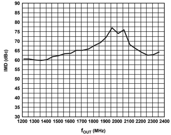
Figure 40. IMD in Mix Mode vs.  $f_{OUT}$  @ 2.4 GSPS
