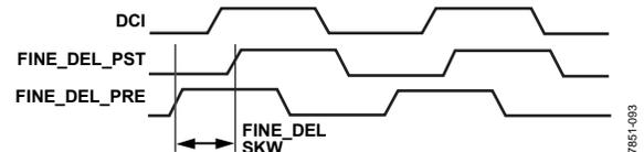
Figure 96. Pre- and Post-Delay Sampling Diagram
