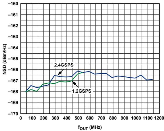
Figure 31. Eight-Tone NSD vs.  $f_{OUT}$  over  $f_{DAC}$
