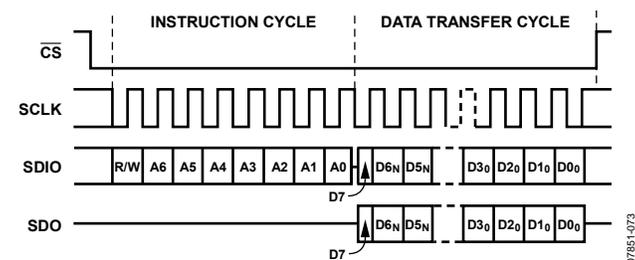
Figure 75. Serial Register Interface Timing, MSB-First Read
