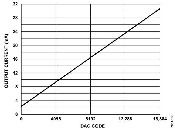
Figure 106. Gain Curve for FSC[9:0] = 1023, DAC OFFSET = 1.932 mA
