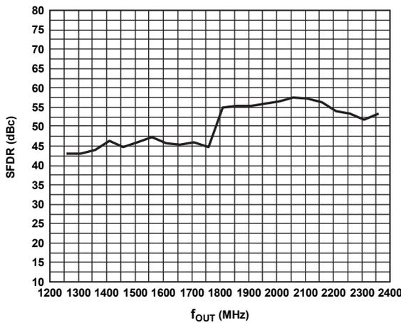
Figure 39. SFDR in Mix Mode vs.  $f_{OUT}$  @ 2.4 GSPS
