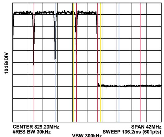
Figure 63. Single-Carrier DOCSIS Close-in ACLR Plot @ 825 MHz
