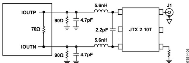
Figure 109. Recommended Transformer Output Stage for DOCSIS Measurements
