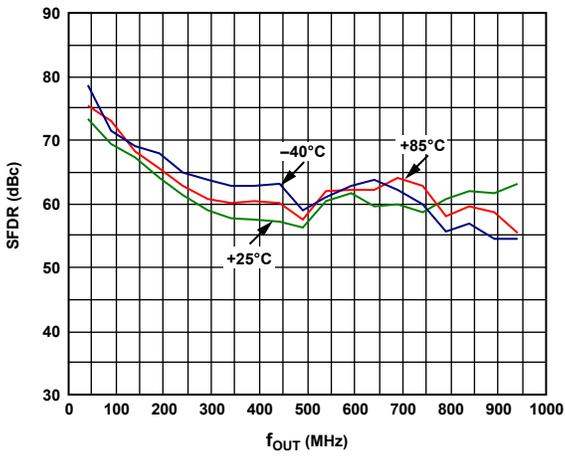
Figure 25. SFDR vs.  $f_{OUT}$  over Temperature @ 2.0 GSPS
