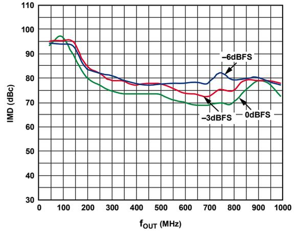
Figure 27. IMD vs.  $f_{OUT}$  over DIGFS @ 2.0 GSPS
