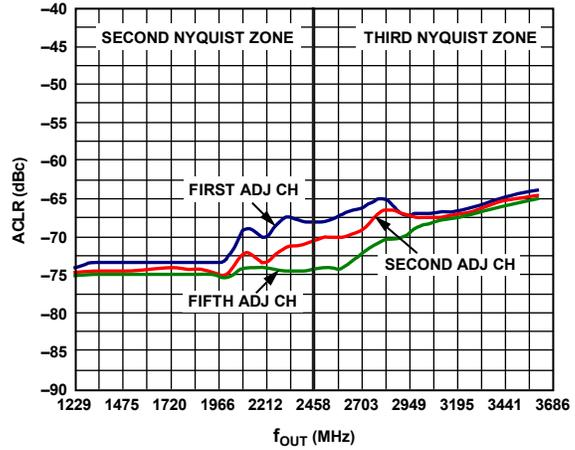
Figure 41. Single-Carrier WCDMA ACLR vs.  $f_{OUT}$  @ 2457.6 MSPS
