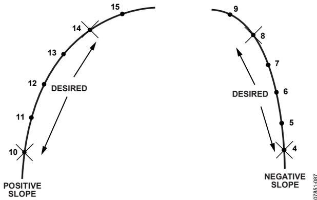
Figure 90. Valid Positive and Negative Slope Phase Examples
