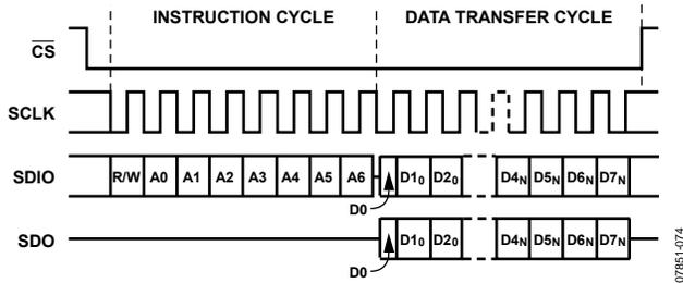
Figure 77. Serial Register Interface Timing, LSB-First Read
