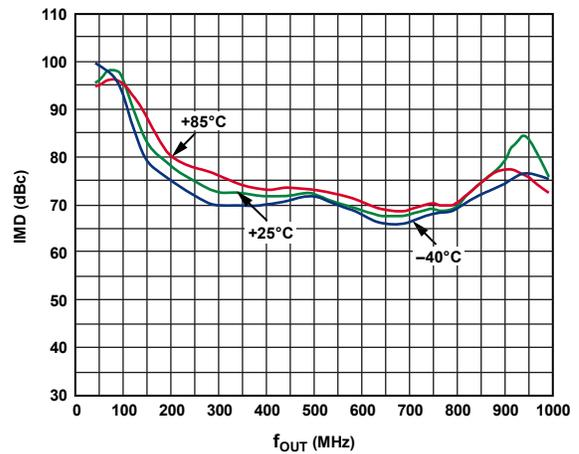
Figure 29. IMD vs.  $f_{OUT}$  over Temperature @ 2.0 GSPS
