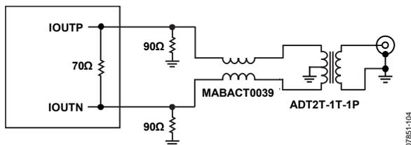
Figure 107. Recommended Transformer Output Stage for Normal Mode
