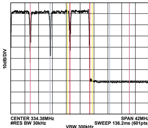
Figure 60. Single-Carrier DOCSIS Close-in ACLR Plot @ 325 MHz
