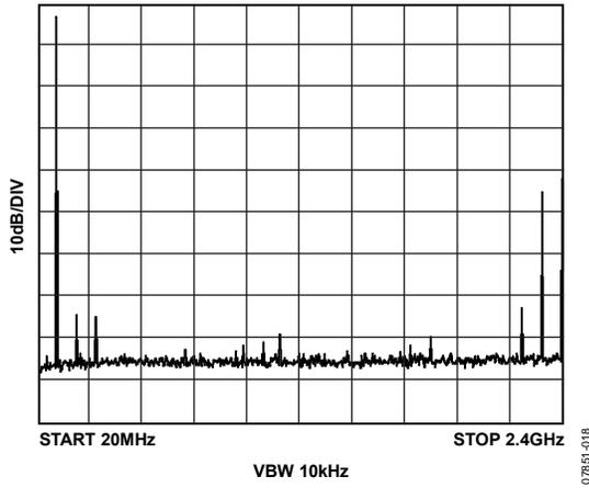
Figure 18. Single Tone Spectrum @  $f_{OUT} = 91$  MHz,  $f_{DAC} = 2.4$  GSPS
