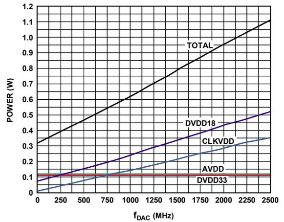
Figure 17. Power Consumption vs.  $f_{DAC}$  @ 25°C
