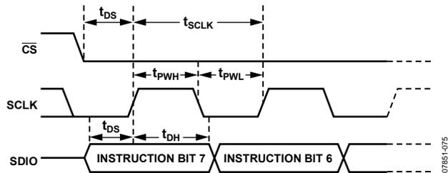
Figure 78. Timing Diagram for an SPI Register Write
