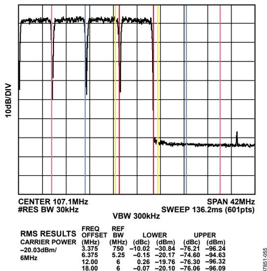
Figure 57. Single-Carrier DOCSIS Close-in ACLR Plot @ 91 MHz
