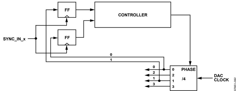
Figure 95. Slave Mode Tracking Mode Block Diagram
