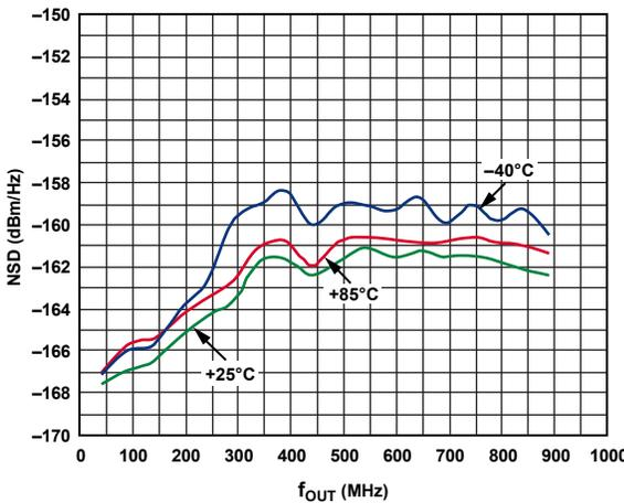
Figure 32. Single-Tone NSD vs.  $f_{OUT}$  over Temperature @ 2.0 GSPS
