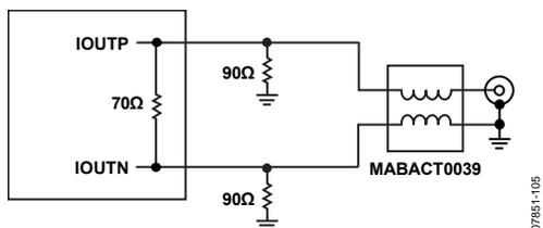
Figure 108. Recommended Transformer Output Stage for Mix Mode
