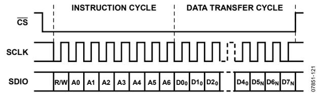
Figure 76. Serial Register Interface Timing, LSB-First Write
