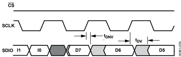
Figure 79. Timing Diagram for an SPI Register Read
