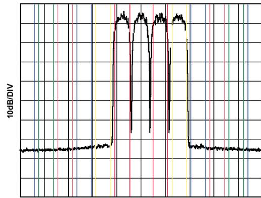
CENTER 355.11MHz SPAN 63.84MHz
