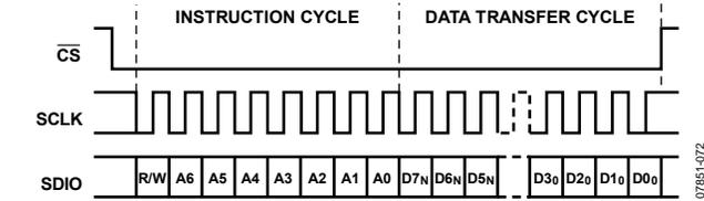
Figure 74. Serial Register Interface Timing, MSB-First Write
