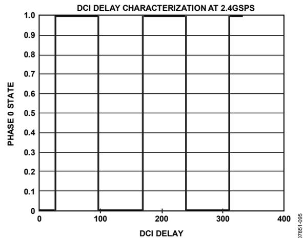
Figure 98. DCI Delay Line Step Size Measurement
