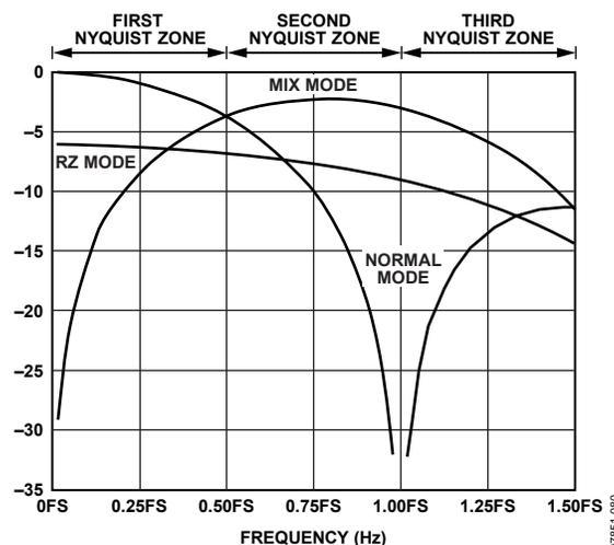
Figure 83. Sinc Roll-Off for Each Analog Operating Mode
