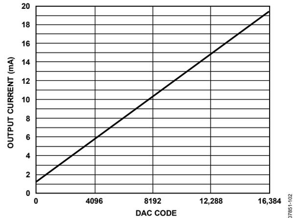
Figure 105. Gain Curve for FSC[9:0] = 512, DAC OFFSET = 1.228 mA
