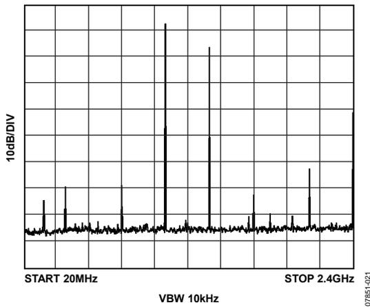
Figure 19. Single Tone Spectrum @  $f_{OUT} = 1091$  MHz,  $f_{DAC} = 2.4$  GSPS
