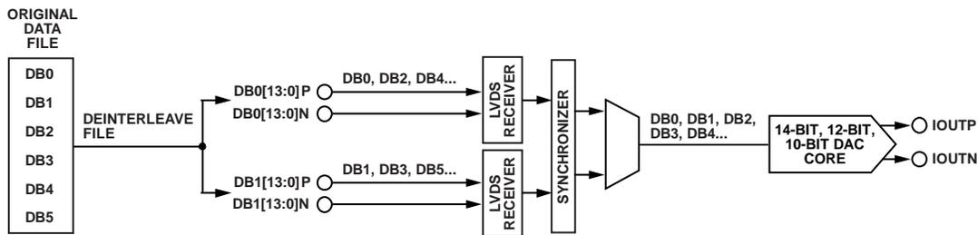
Figure 87. Graphical Representation of How to Present Data to the AD9739
