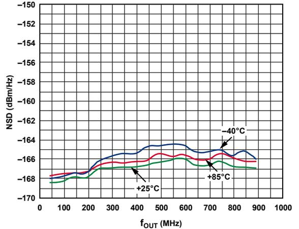
Figure 33. Eight-Tone NSD vs.  $f_{OUT}$  over Temperature @ 2.0 GSPS
