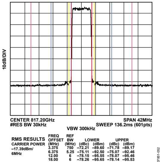
Figure 54. Single-Carrier DOCSIS Close-in ACLR Plot @ 825 MHz
