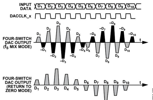
Figure 82. Mix Mode and RZ DAC Waveforms
