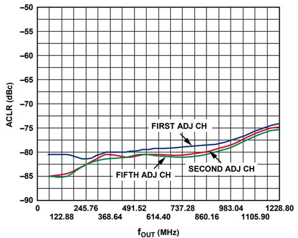
Figure 34. Single-Carrier WCDMA ACLR vs.  $f_{OUT}$  @ 2457.6 MSPS
