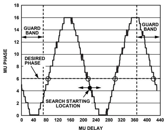
Figure 89. Typical Mu Phase Characteristic Plot @ 2.4 GSPS
