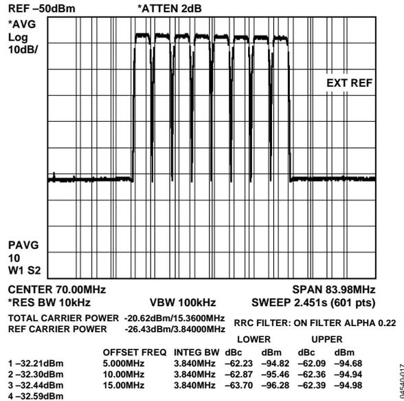
Figure 16. Eight-Carrier WCDMA @ 400 MSPS  $f_{OUT} = 70$  MHz
