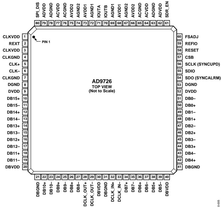
Figure 5. Pin Configuration
