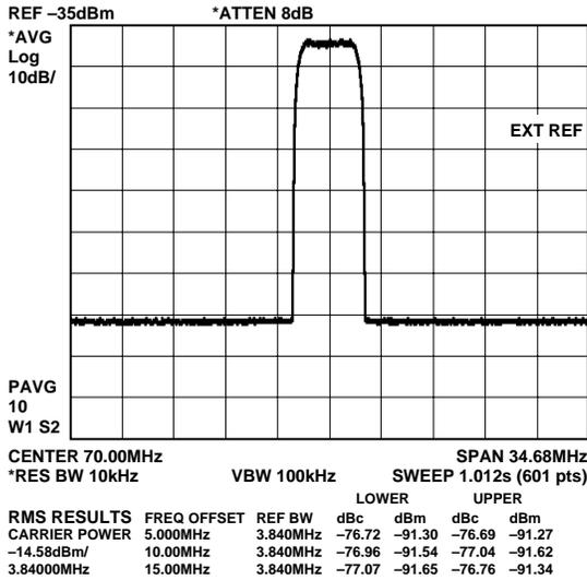
Figure 13. One-Carrier WCDMA @ 400 MSPS  $f_{OUT} = 70$  MHz
