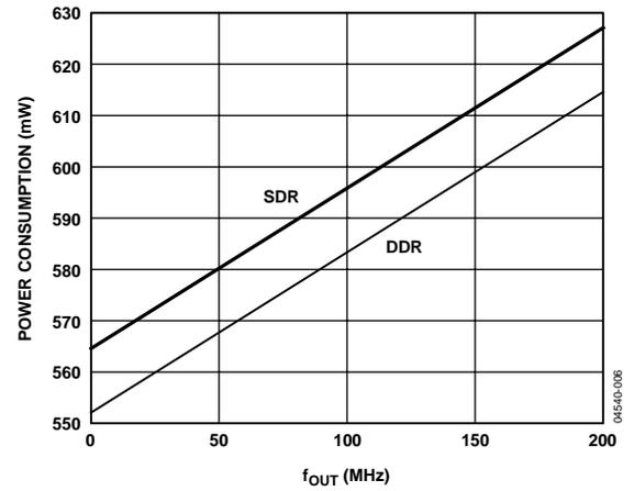
Figure 9. Power Consumption vs.  $f_{OUT}$  @ 400 MSPS
