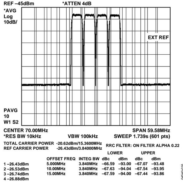
Figure 15. Four-Carrier WCDMA @ 400 MSPS  $f_{OUT} = 70$  MHz
