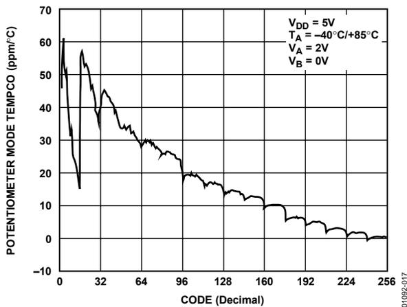
Figure 17.  $\Delta V_{WB}/\Delta T$  Potentiometer Mode Tempco
