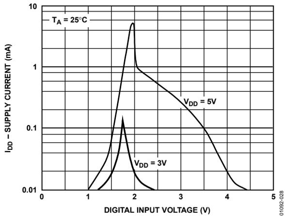
Figure 28. Supply Current vs. Digital Input Voltage
