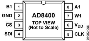
Figure 6. AD8400 Pin Configuration
