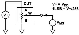
Figure 37. Potentiometer Divider Nonlinearity Error (INL, DNL)
