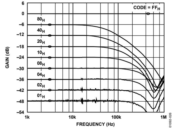
Figure 26. 100 kΩ Gain vs. Frequency vs. Code
