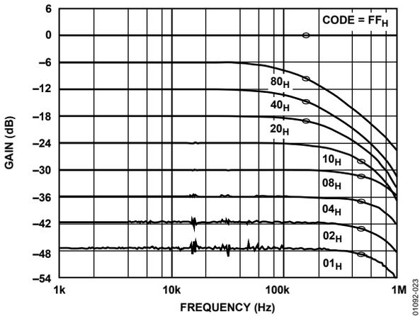
Figure 23. 50 kΩ Gain vs. Frequency vs. Code
