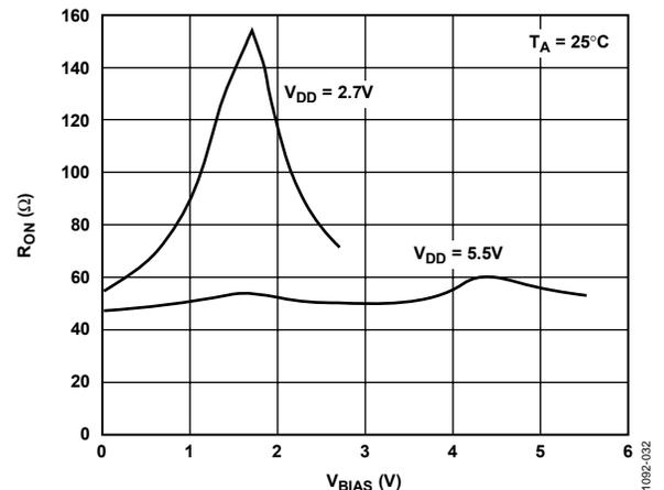
Figure 32. AD8403 Incremental Wiper On Resistance vs.  $V_{DD}$
