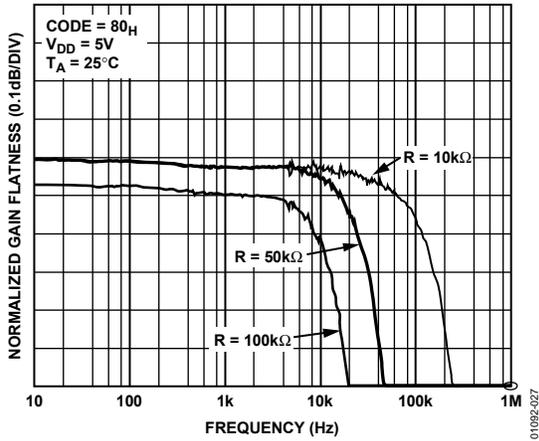
Figure 27. Normalized Gain Flatness vs. Frequency
