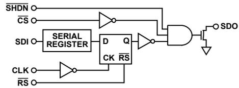
Figure 50. Detailed SDO Output Schematic of the AD8403
