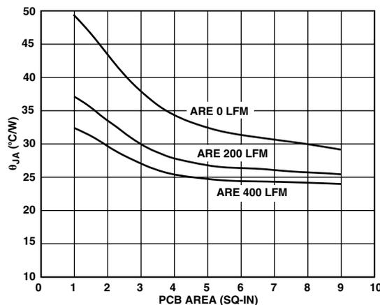
Figure 44. Junction-to-Ambient Thermal Resistance vs. PCB Area
