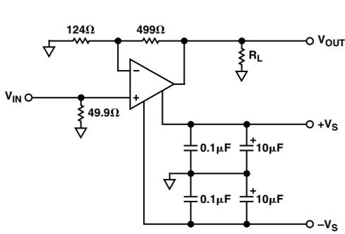
Figure 3. Single-Ended Test Circuit;  $G = +5$
