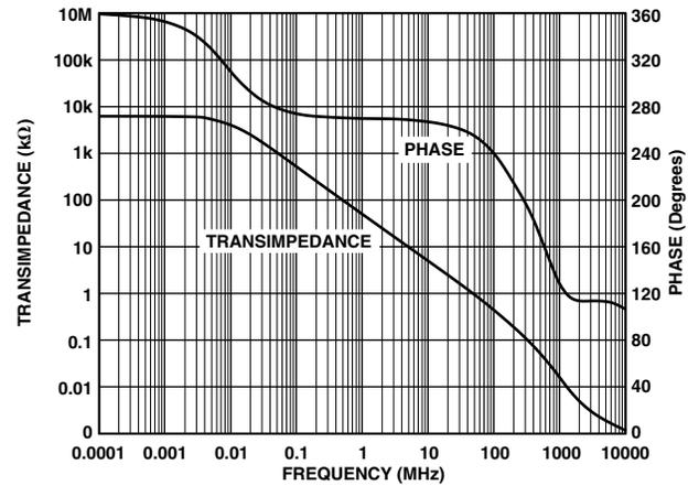
Figure 30. Open-Loop Transimpedance and Phase vs. Frequency
