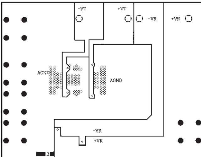
Figure 49. Power/Ground Plane
