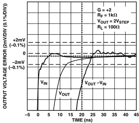
Figure 28. Settling Time 0.1%;  $V_S = \pm 12 V$
