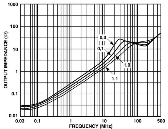
Figure 32. Output Impedance vs. Frequency @ PWDN1, PWDN0 Codes
