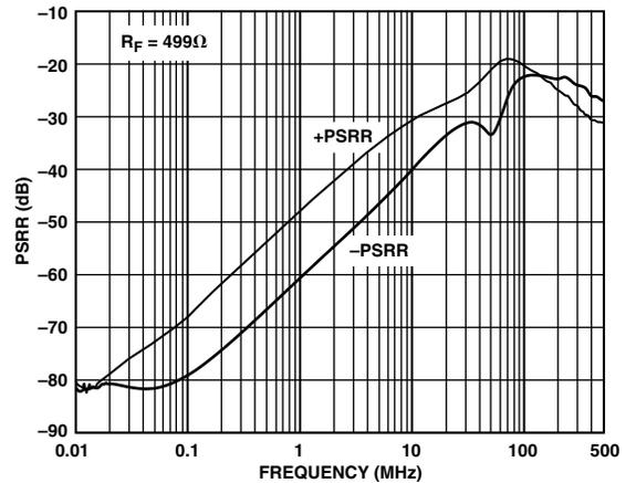
Figure 26. PSRR vs. Frequency;  $V_S = \pm 12\text{ V}$
