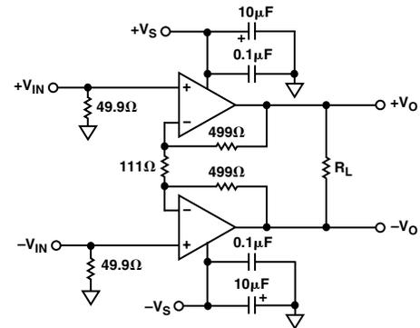
Figure 6. Differential Test Circuit;  $G = +10$
