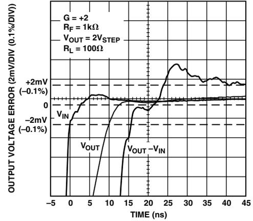
Figure 31. Settling Time 0.1%;  $V_S = \pm 6 V$
