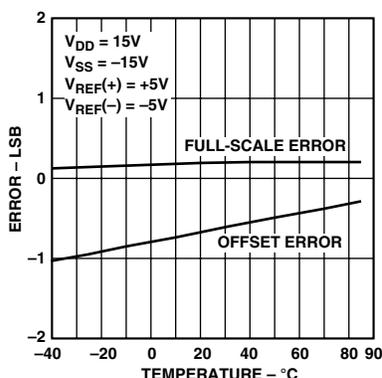
Figure 6. Offset and Full-Scale Error vs. Temperature
