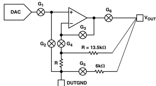
Figure 13. Block Diagram of AD7836 Output Stage
