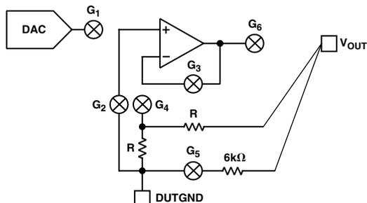
Figure 14. Output Stage with  $V_{DD} < 10\text{ V}$
