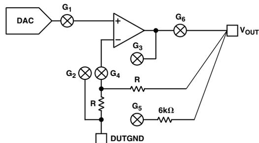
Figure 16. Output Stage After  $\overline{\text{CLR}}$  Is Taken High
