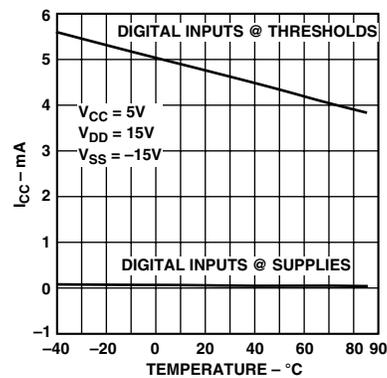
Figure 7.  $I_{CC}$  vs. Temperature
