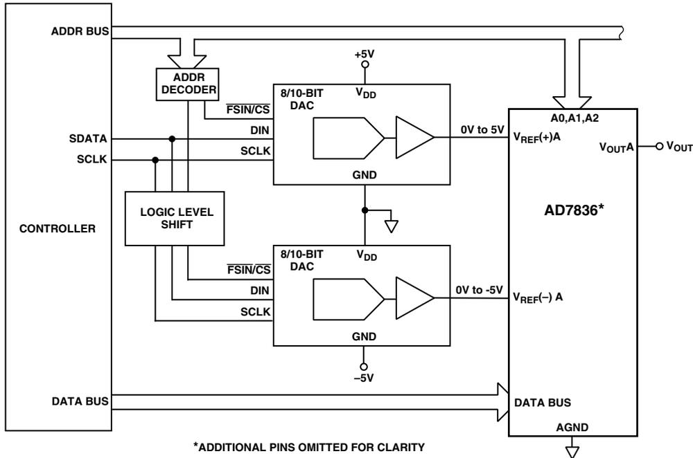
Figure 22. Programmable Reference Generation for the AD7836
