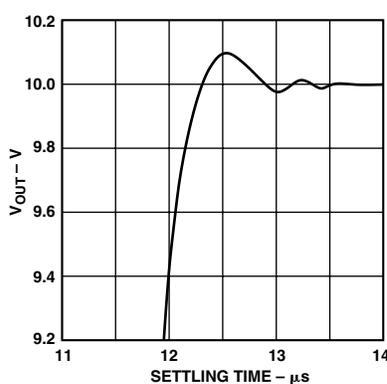
Figure 9. Settling Time (+)
