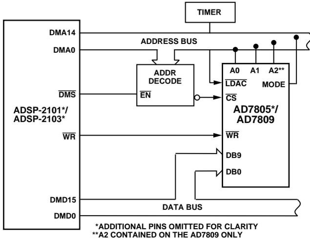
Figure 38. AD7805/AD7809-ADSP-2101/ADSP-2103 Interface
