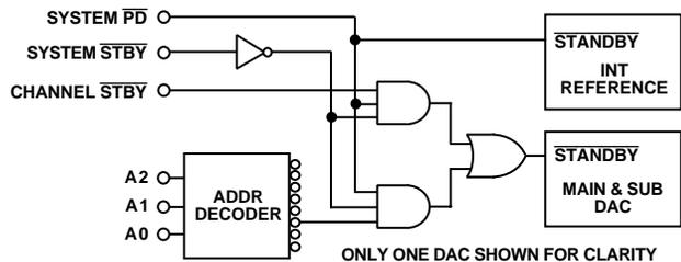
Figure 21. Implementation of Power-Down and Standby Functions
