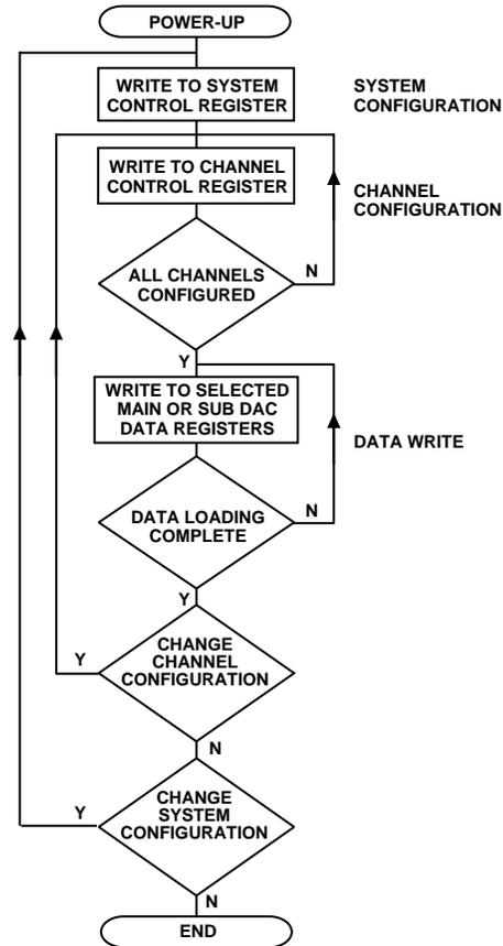
Figure 10. Flowchart for Controlling the DAC Following Power-Up
