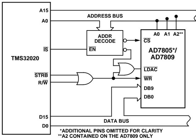
Figure 39. AD7805/AD7809-TMS32020 Interface
