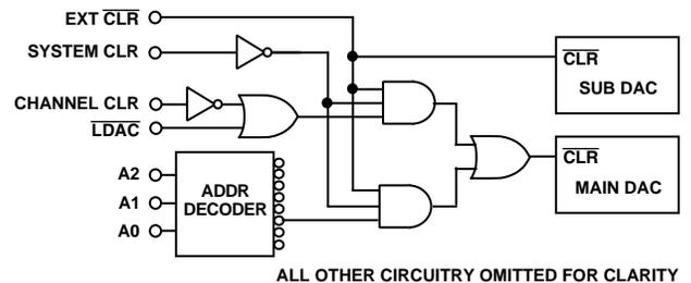
Figure 20.  $\overline{CLR}$  Functions for Main and Sub DACs
