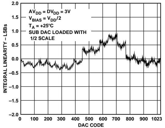
Figure 33. Integral Linearity with 3 V Operation
