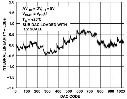
Figure 32. Integral Linearity with 5 V Operation
