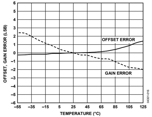
Figure 19. Offset and Gain Error vs. Temperature
