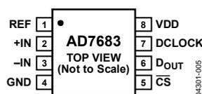
Figure 6. 8-Lead MSOP and QFN (LFCSP) Pin Configuration
