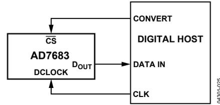
Figure 25. Connection Diagram
