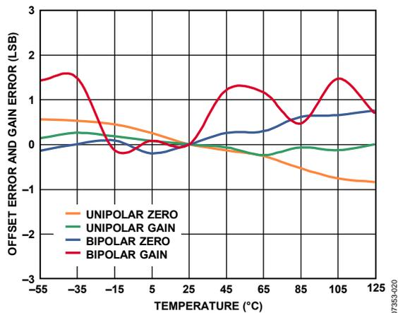
Figure 20. Offset and Gain Errors vs. Temperature
