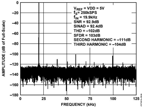
Figure 8. 20 kHz FFT, VREF = VDD = 5 V
