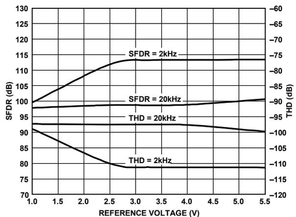
Figure 16. SFDR and THD vs. Reference Voltage
