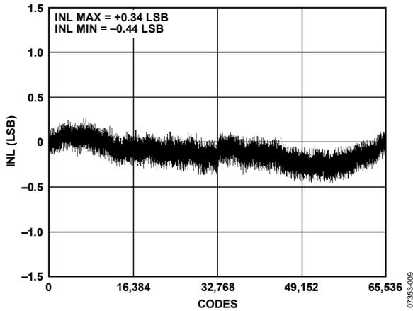
Figure 6. Integral Nonlinearity vs. Code, VREF = VDD = 5 V
