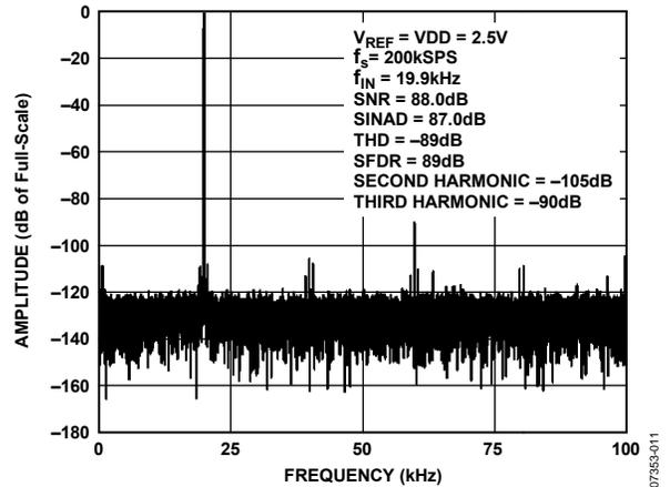
Figure 11. 20 kHz FFT, VREF = VDD = 2.5 V
