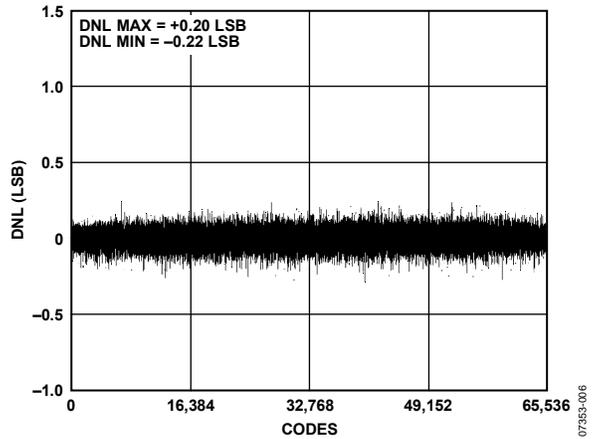
Figure 9. Differential Nonlinearity vs. Code, VREF = VDD = 5 V
