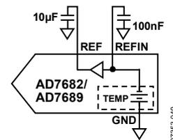
Figure 31. 2.5 V or 4.096 V Internal Reference Connection
