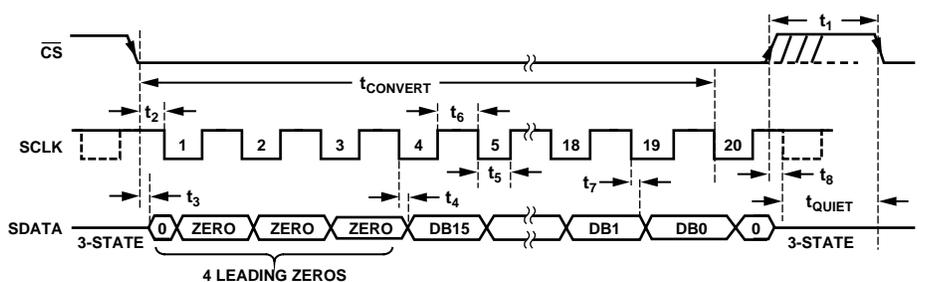
Figure 21. AD7680 Serial Interface Timing Diagram—20 SCLK Transfer
