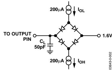
Figure 2. Load Circuit for Digital Output Timing Specification
