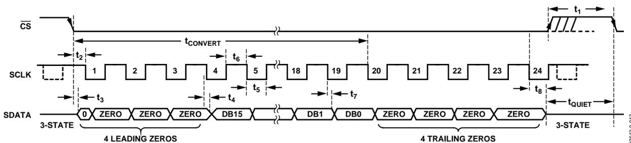
Figure 20. AD7680 Serial Interface Timing Diagram—24 SCLK Transfer
