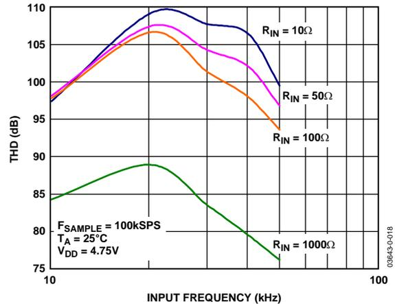
Figure 8. AD7680 THD vs. Analog Input Frequency for Various Source Impedances
