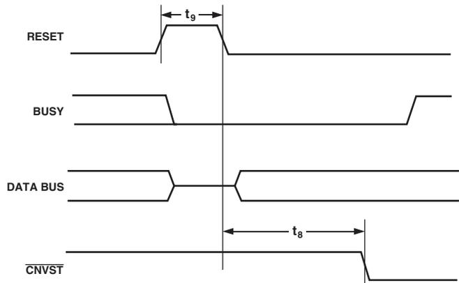
Figure 12. RESET Timing
