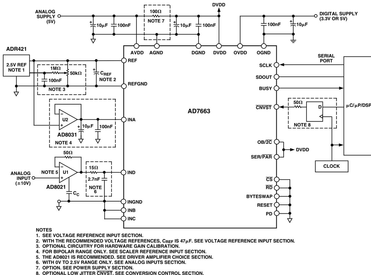
Figure 5. Typical Connection Diagram ( $\pm 10$  V Range Shown)
