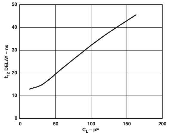
TPC 12. Typical Delay vs. Load Capacitance,  $C_L$
