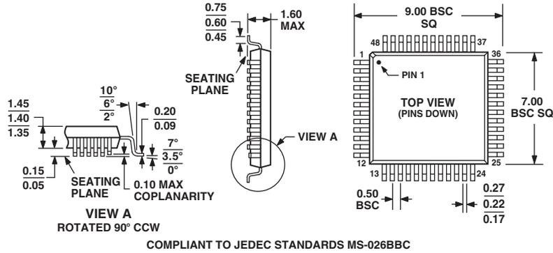
48-Lead Lead Frame Chip Scale Package [LFCSP]
