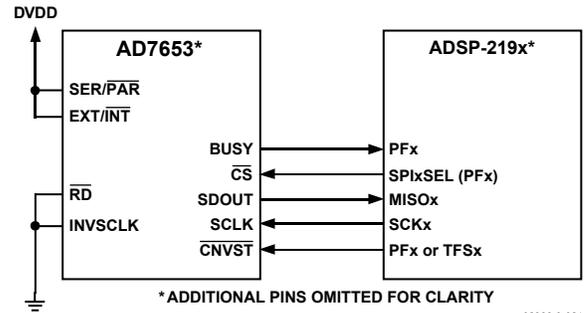
Figure 37. Interfacing the AD7653 to an SPI Interface
