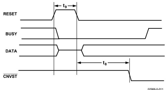
Figure 27. RESET Timing
