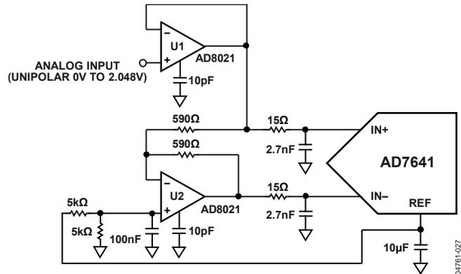
Figure 26. Single-Ended-to-Differential Driver Circuit (Internal Reference Buffer Used)
