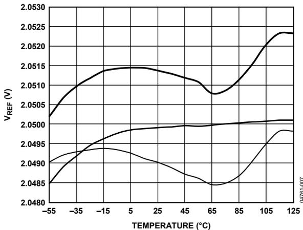
Figure 7. Typical Reference Voltage Output vs. Temperature (3 Units)
