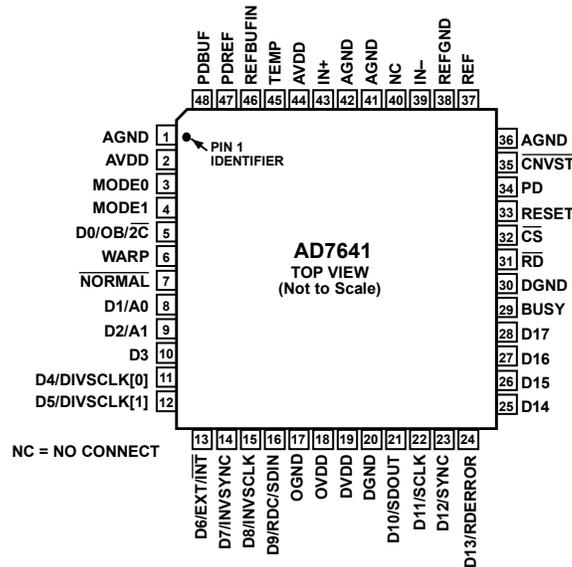
Figure 4. Pin Configuration
