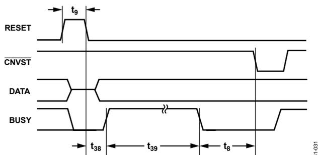
Figure 30. RESET Timing
