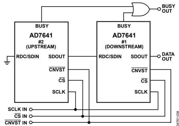
Figure 37. Two AD7641 Devices in a Daisy-Chain Configuration
