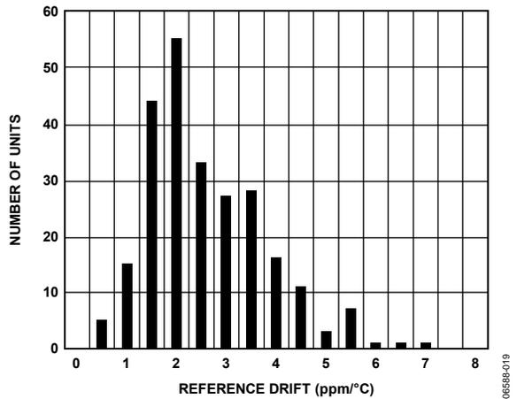
Figure 19. Reference Voltage Temperature Coefficient Distribution (247 Devices)
