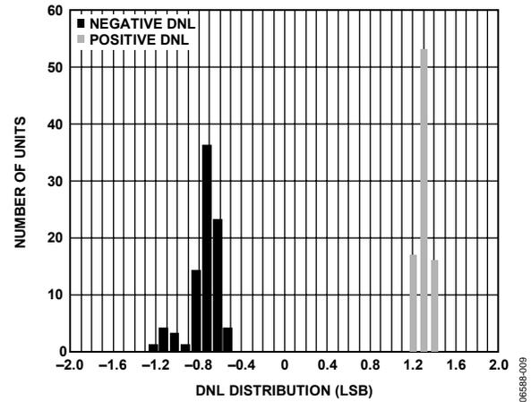
Figure 9. Differential Nonlinearity Distribution, Bipolar 5 V Range (86 Devices)
