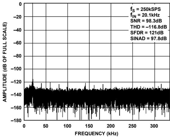
Figure 11. FFT 20 kHz, Bipolar 5 V Range, Internal Reference
