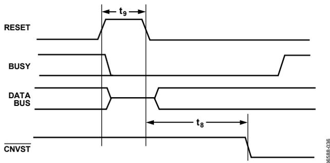
Figure 36. RESET Timing
