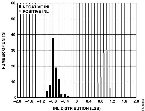
Figure 6. Integral Nonlinearity Distribution, Unipolar 10 V Range (86 Devices)
