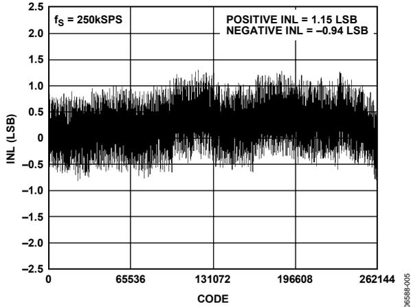
Figure 5. Integral Nonlinearity vs. Code, Bipolar 10 V Range
