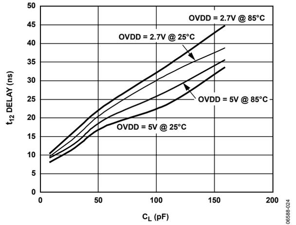
Figure 24. Typical Delay vs. Load Capacitance  $C_L$
