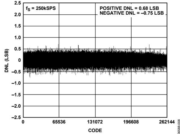
Figure 8. Differential Nonlinearity vs. Code, Bipolar 10 V Range
