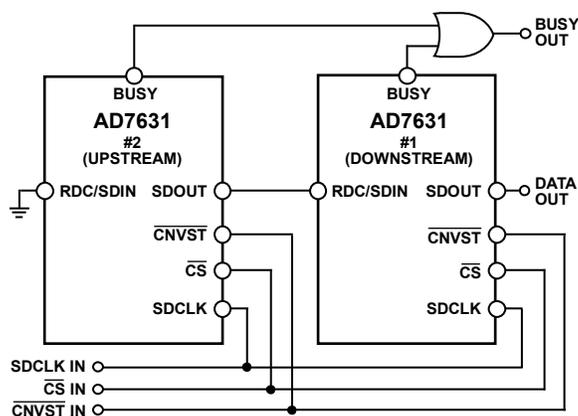
Figure 43. Two AD7631 Devices in a Daisy-Chain Configuration
