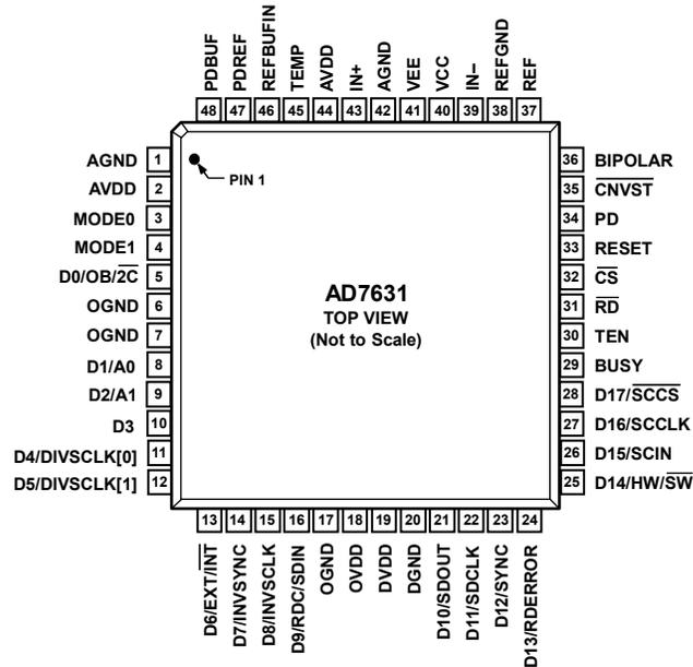
Figure 4. Pin Configuration
