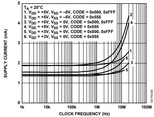
Figure 20. AD7398 Supply Current vs. Clock Frequency
