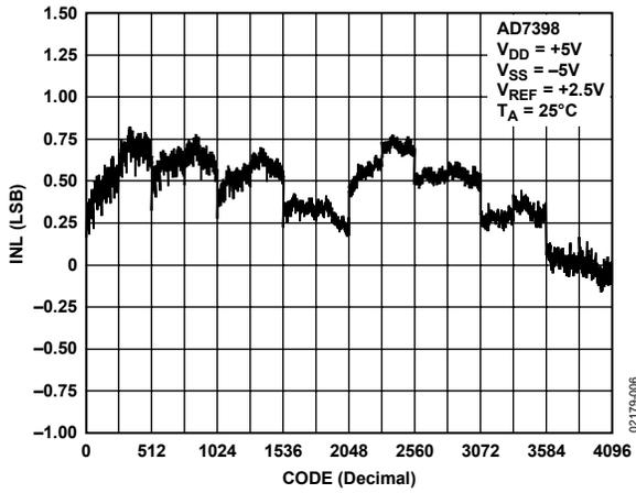
Figure 6. AD7398 INL vs. Code ( $T_A = 25^\circ\text{C}$ )
