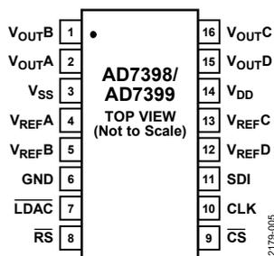
Figure 5. Pin Configuration
