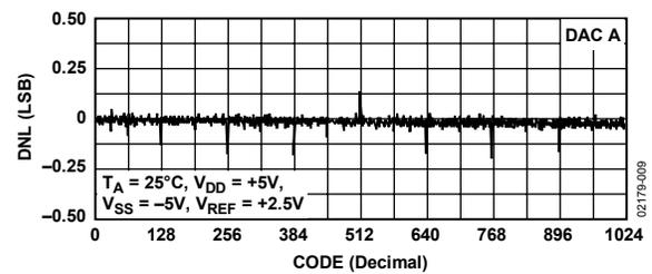
Figure 9. AD7399 DNL vs. Code ( $T_A = 25^\circ\text{C}$ )
