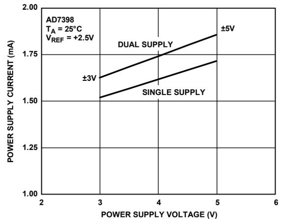
Figure 21. AD7398 Supply Current vs. Supply Voltage
