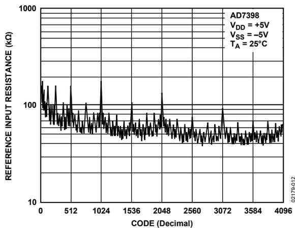
Figure 12. AD7398 Reference Input Resistance vs. Code
