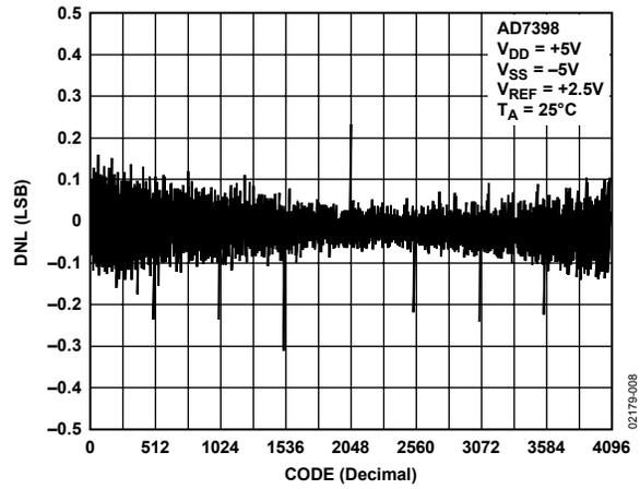
Figure 8. AD7398 DNL vs. Code ( $T_A = 25^\circ\text{C}$ )
