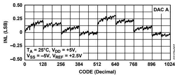
Figure 7. AD7399 INL vs. Code ( $T_A = 25^\circ\text{C}$ )
