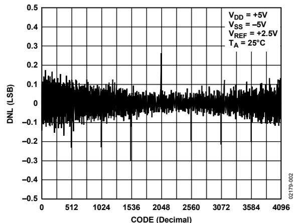
Figure 2. AD7398 DNL vs. Code ( $T_A = 25^{\circ}\text{C}$ )
