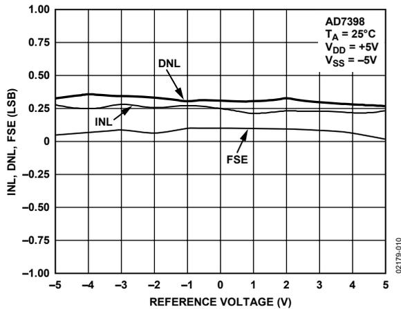
Figure 10. AD7398 INL, DNL, FSE vs. Reference Voltage
