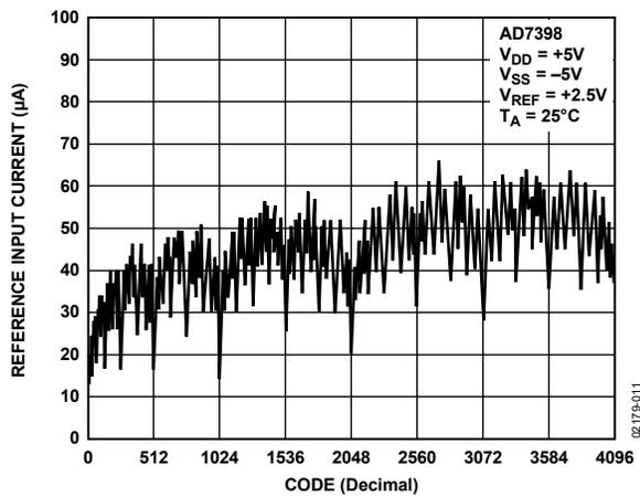
Figure 11. AD7398 Reference Input Current vs. Code
