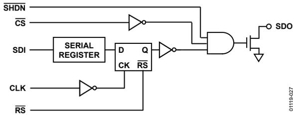
Figure 27. Detailed SDO Output Schematic of the AD7376
