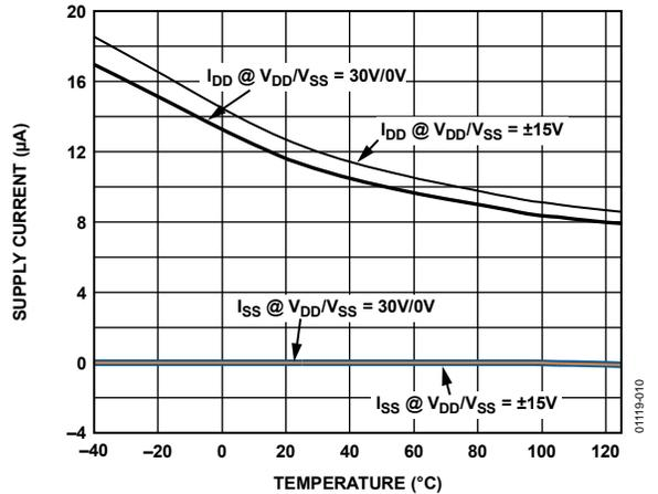
Figure 10. Supply Current ( $I_{DD}$ ,  $I_{SS}$ ) vs. Temperature
