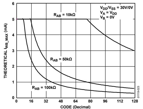
Figure 23. Theoretical Maximum Current vs. Code
