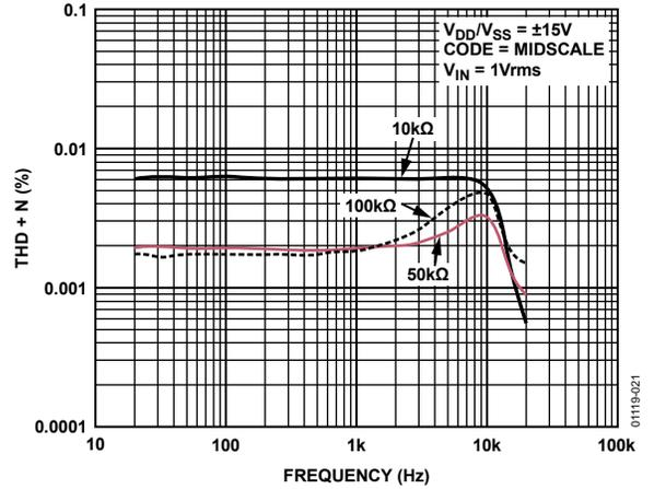
Figure 21. Total Harmonic Distortion Plus Noise vs. Frequency
