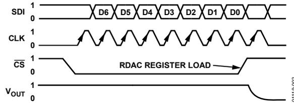
Figure 2. AD7376 3-Wire Digital Interface Timing Diagram
