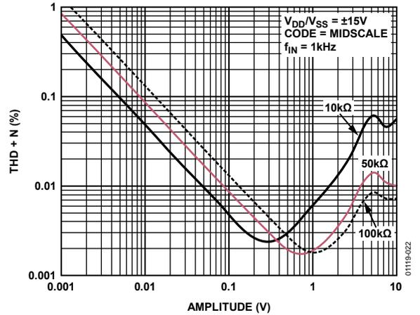
Figure 22. Total Harmonic Distortion Plus Noise vs. Amplitude
