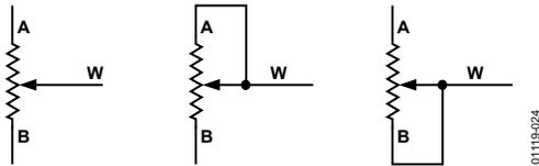
Figure 24. Rheostat Mode Configuration
