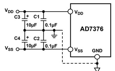
Figure 31. Power Supply Bypassing
