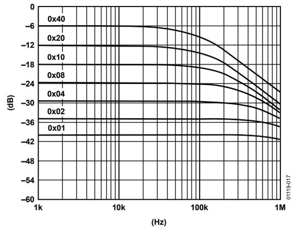
Figure 17. 50 kΩ Gain vs. Frequency vs. Code
