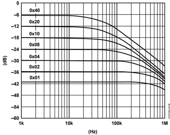
Figure 18. 100 kΩ Gain vs. Frequency vs. Code
