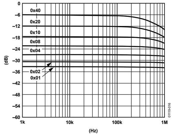
Figure 16. 10 kΩ Gain vs. Frequency vs. Code
