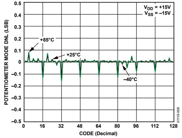
Figure 9. Potentiometer Divider Differential Nonlinearity Error vs. Code
