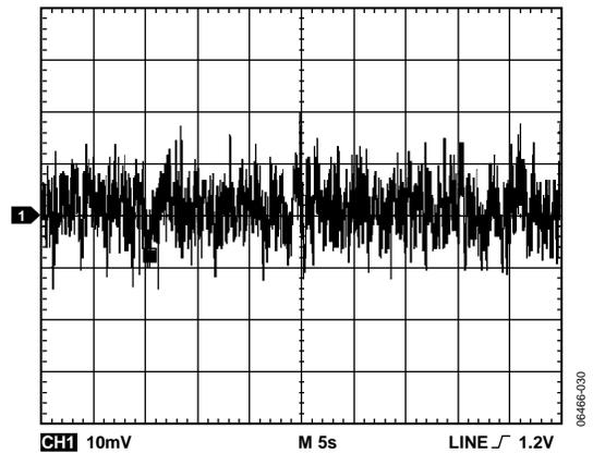
Figure 35. REFOUT Output Noise (0.1 Hz to 10 Hz Bandwidth)
