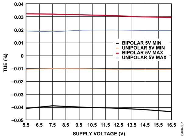
Figure 19. AD5752R Total Unadjusted Error vs. Supply Voltage
