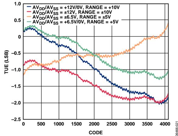
Figure 39. AD5722R Total Unadjusted Error vs. Code
