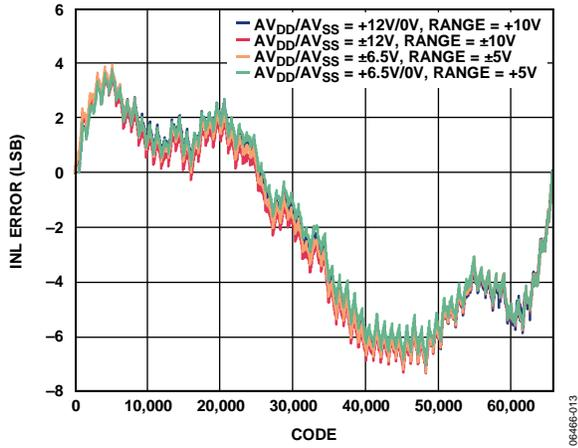
Figure 6. AD5752R Integral Nonlinearity Error vs. Code
