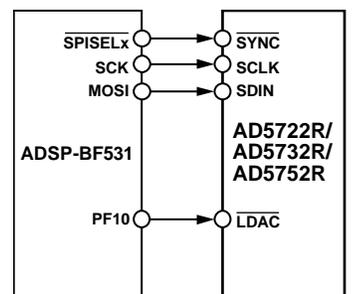
Figure 50. AD5722R/AD5732R/AD5752R-to-Blackfin Interface
