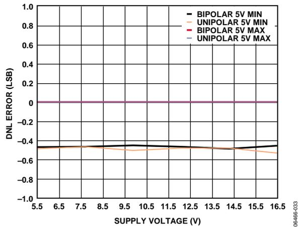
Figure 17. AD5752R Differential Nonlinearity Error vs. Supply Voltage
