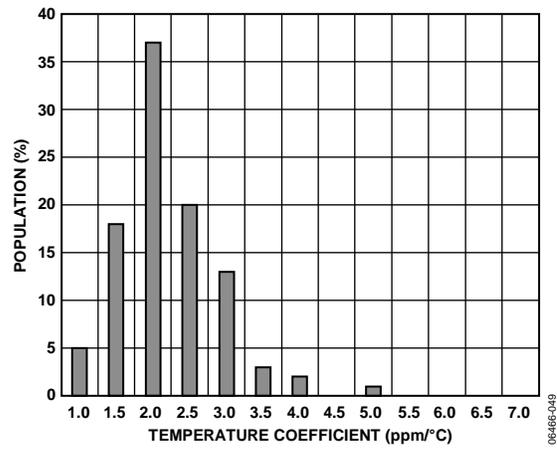
Figure 40. Reference Output TC (-40°C to +85°C)
