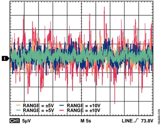
Figure 30. Peak-to-Peak Noise, 0.1 Hz to 10 Hz Bandwidth
