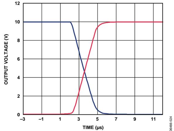
Figure 27. Full-Scale Settling Time, +10 V Range
