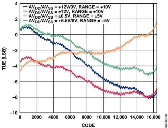
Figure 38. AD5732R Total Unadjusted Error vs. Code
