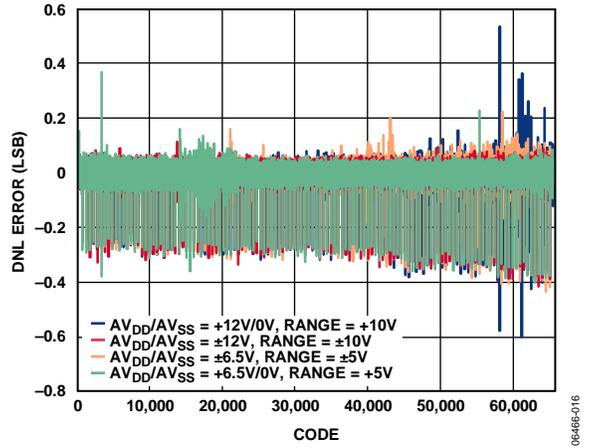
Figure 9. AD5752R Differential Nonlinearity Error vs. Code
