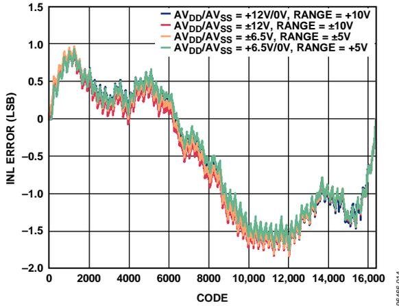
Figure 7. AD5732R Integral Nonlinearity Error vs. Code
