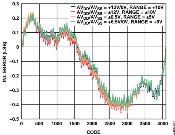
Figure 8. AD5722R Integral Nonlinearity Error vs. Code
