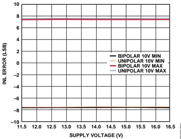
Figure 14. AD5752R Integral Nonlinearity Error vs. Supply Voltage
