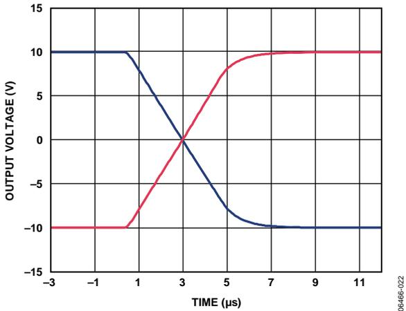
Figure 25. Full-Scale Settling Time, ±10 V Range
