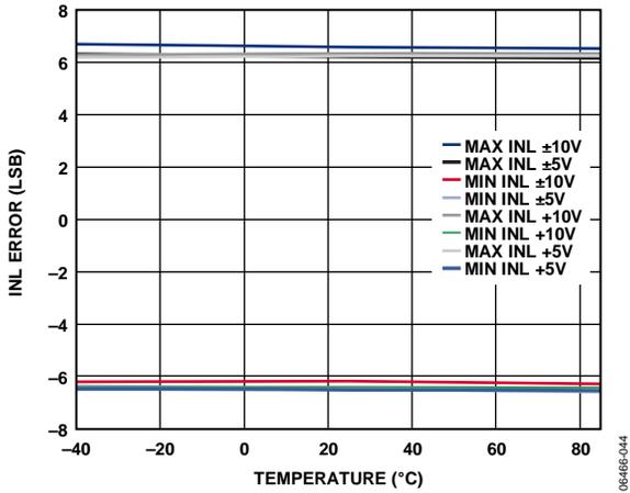
Figure 12. AD5752R Integral Nonlinearity Error vs. Temperature
