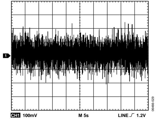
Figure 34. REFOUT Output Noise (100 kHz Bandwidth)
