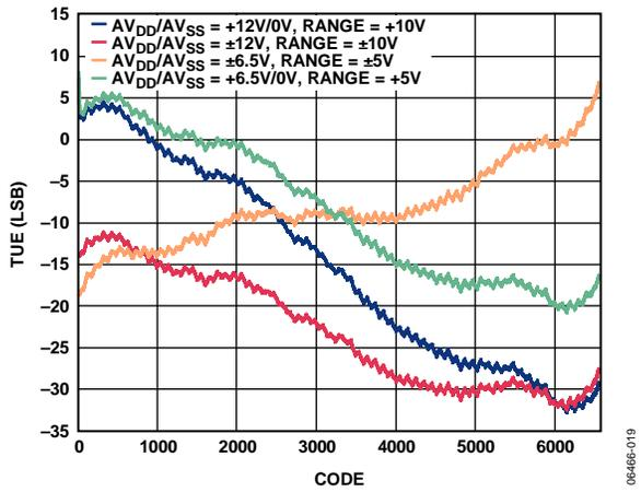
Figure 37. AD5752R Total Unadjusted Error vs. Code
