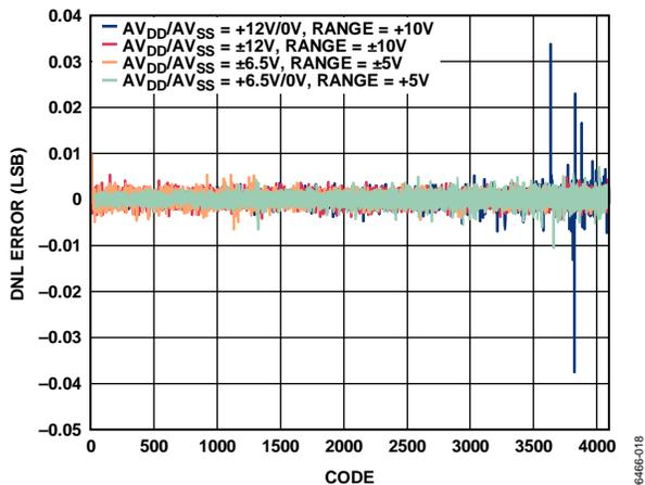
Figure 11. AD5722R Differential Nonlinearity Error vs. Code
