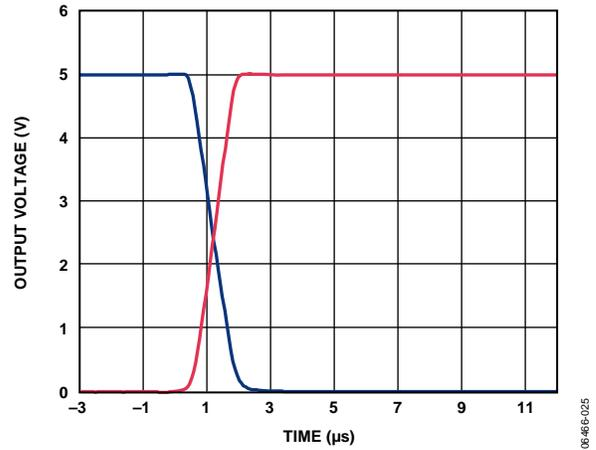
Figure 28. Full-Scale Settling Time, +5 V Range
