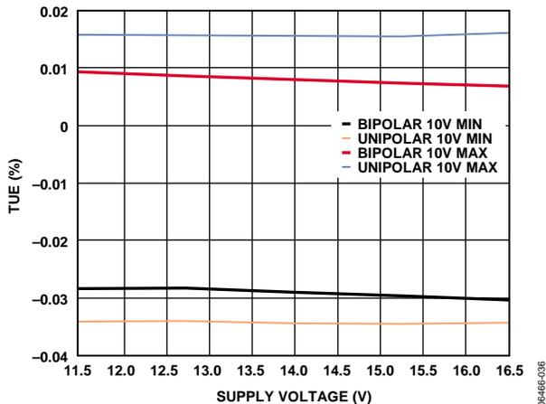
Figure 18. AD5752R Total Unadjusted Error vs. Supply Voltage
