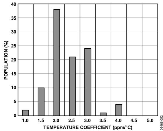
Figure 41. Reference Output TC (0°C to 85°C)
