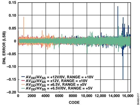
Figure 10. AD5732R Differential Nonlinearity Error vs. Code
