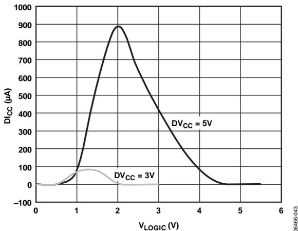
Figure 23. Digital Current vs. Logic Input Voltage
