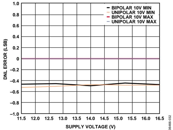
Figure 15. AD5752R Differential Nonlinearity Error vs. Supply Voltage
