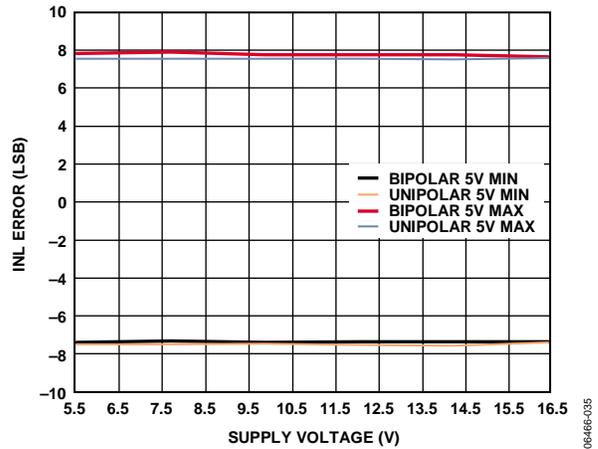
Figure 16. AD5752R Integral Nonlinearity Error vs. Supply Voltage
