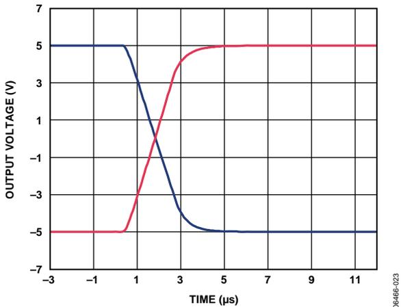
Figure 26. Full-Scale Settling Time, ±5 V Range
