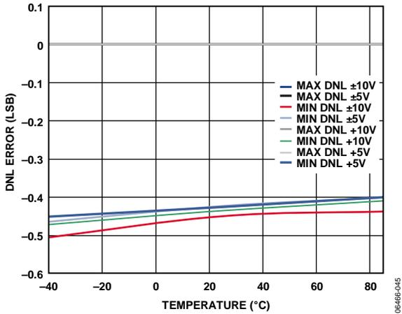
Figure 13. AD5752R Differential Nonlinearity Error vs. Temperature
