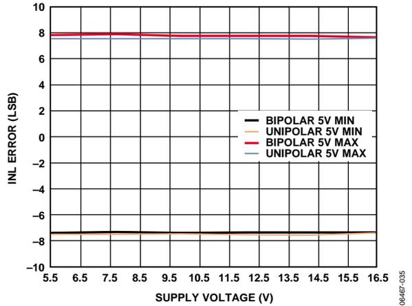
Figure 15. AD5752 Integral Nonlinearity Error vs. Supply Voltage
