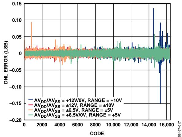
Figure 10. AD5732 Differential Nonlinearity Error vs. Code
