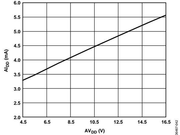
Figure 21. Supply Current vs. Supply Voltage (Single Supply)
