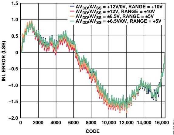
Figure 7. AD5732 Integral Nonlinearity Error vs. Code
