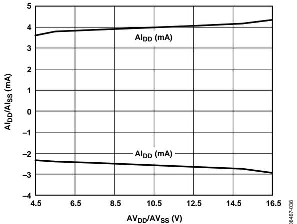
Figure 20. Supply Current vs. Supply Voltage (Dual Supply)
