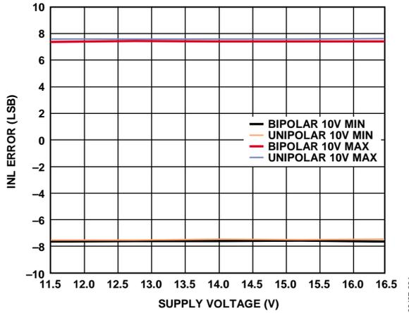
Figure 14. AD5752 Integral Nonlinearity Error vs. Supply Voltage
