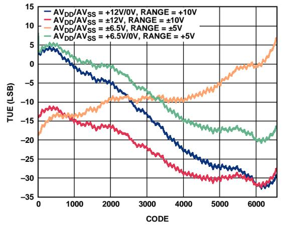
Figure 35. AD5752 Total Unadjusted Error vs. Code
