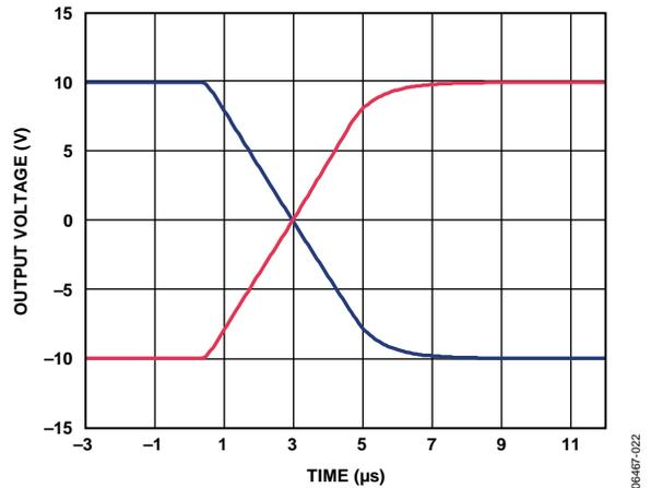
Figure 27. Full-Scale Settling Time,  $\pm 10V$  Range
