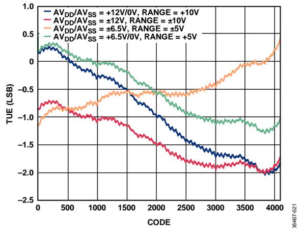
Figure 37. AD5722 Total Unadjusted Error vs. Code
