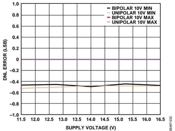
Figure 16. AD5752 Differential Nonlinearity Error vs. Supply Voltage
