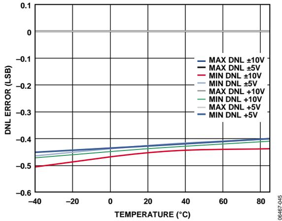
Figure 13. AD5752 Differential Nonlinearity Error vs. Temperature
