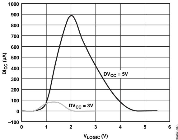
Figure 25. Digital Current vs. Logic Input Voltage
