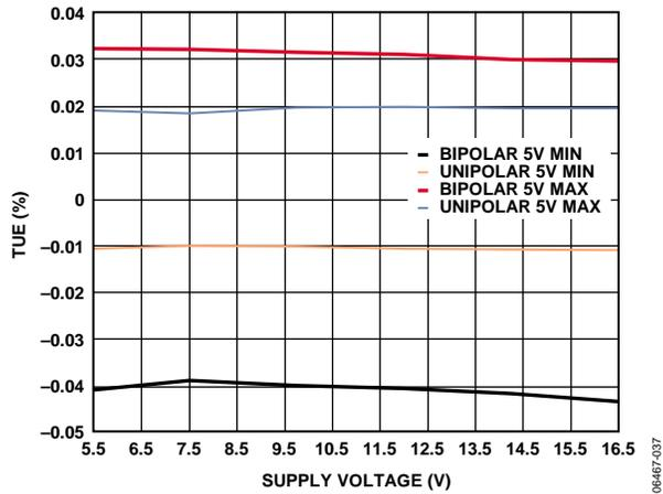
Figure 19. AD5752 Total Unadjusted Error vs. Supply Voltage
