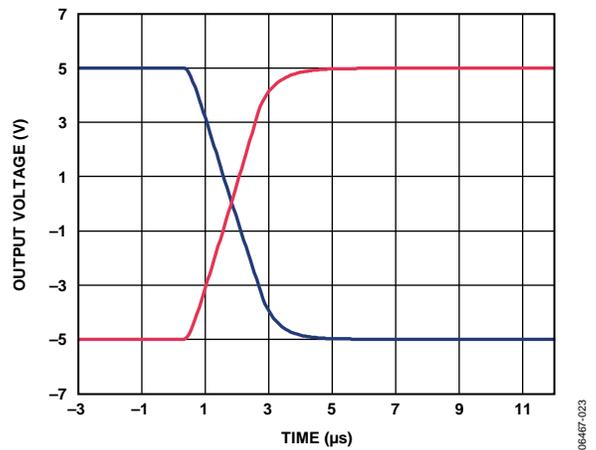
Figure 28. Full-Scale Settling Time,  $\pm 5V$  Range
