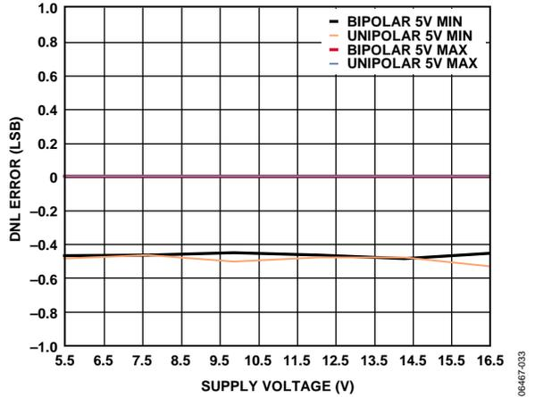
Figure 17. AD5752 Differential Nonlinearity Error vs. Supply Voltage
