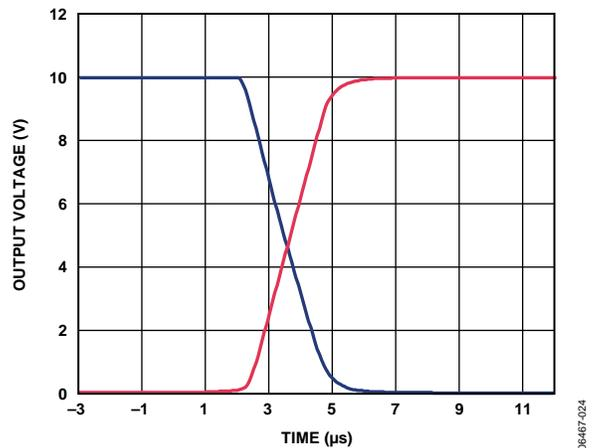
Figure 29. Full-Scale Settling Time, +10 V Range
