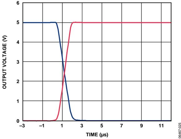
Figure 30. Full-Scale Settling Time, +5 V Range
