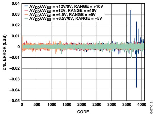
Figure 11. AD5722 Differential Nonlinearity Error vs. Code
