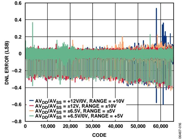
Figure 9. AD5752 Differential Nonlinearity Error vs. Code
