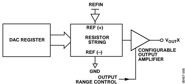
Figure 38. DAC Architecture Block Diagram
