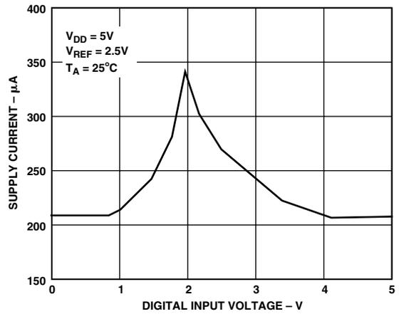
TPC 9. Supply Current vs. Digital Input Voltage
