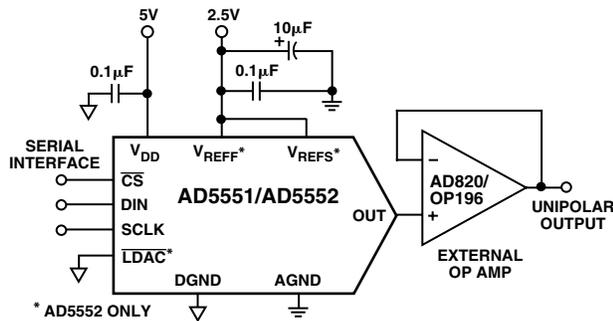
Figure 3. Unipolar Output
