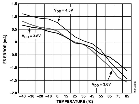
Figure 16. Full-Scale Error vs. Temperature vs. Supply
