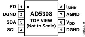
Figure 3. 8-Lead LFSCP Pin Configuration
