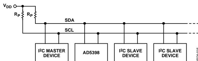
Figure 18. Typical I<sup>2</sup>C Bus
