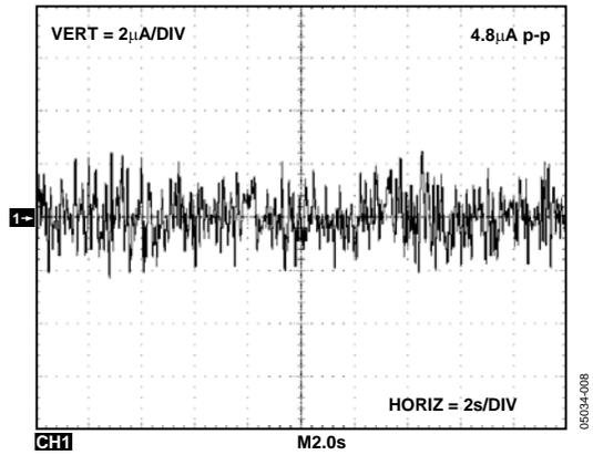
Figure 10. 0.1 Hz to 10 Hz Noise Plot ( $V_{DD} = 3.6 V$ )
