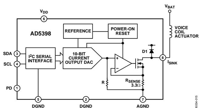
Figure 17. Block Diagram Showing Connection to Voice Coil
