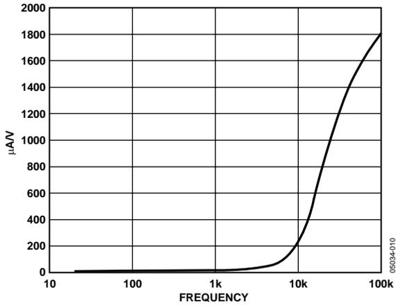
Figure 12. AC Power Supply Rejection ( $V_{DD} = 3.6\text{ V}$ )
