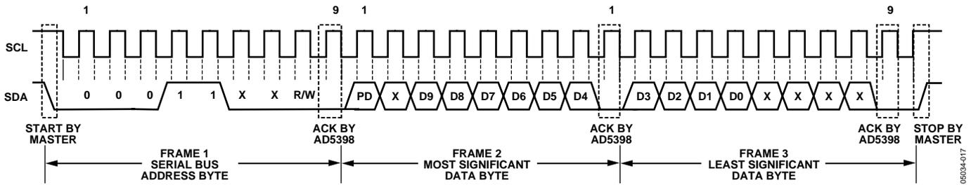
Figure 19. Write Operation
