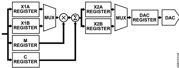
Figure 18. Data Registers Associated with Each DAC Channel
