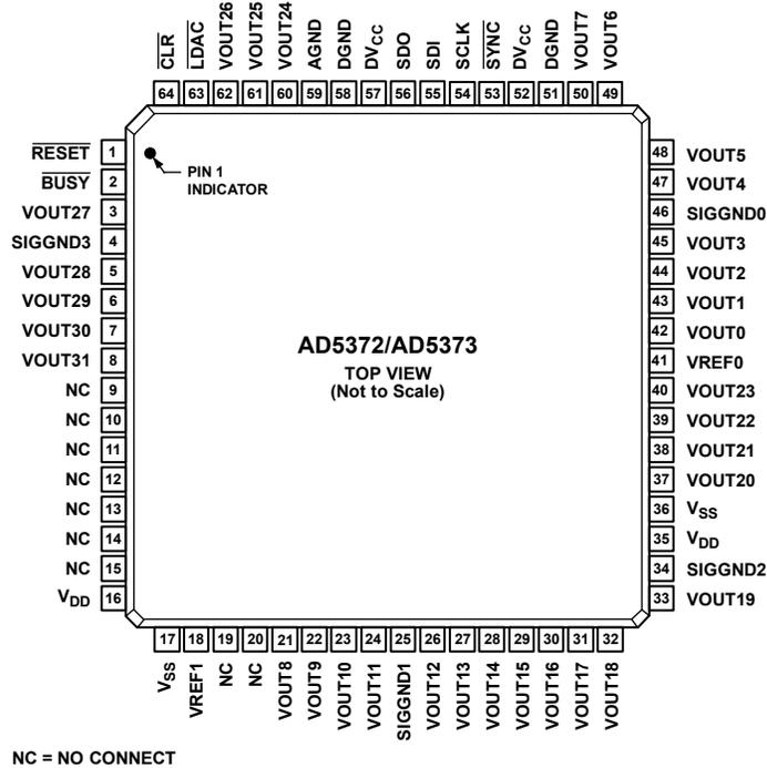
Figure 7. Pin Configuration
