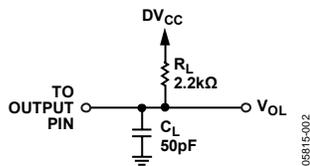
Figure 2. Load Circuit for  $\overline{\text{BUSY}}$  Timing Diagram
