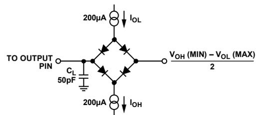
Figure 3. Load Circuit for SDO Timing Diagram
