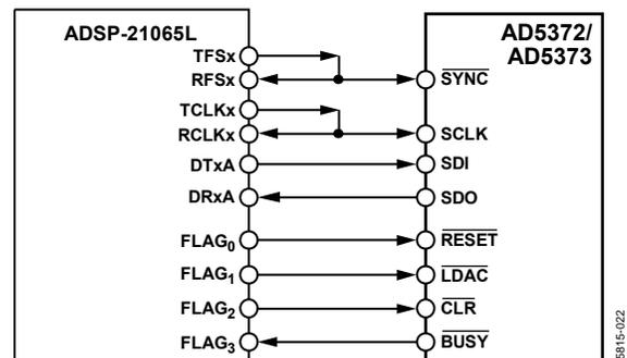
Figure 22. Interfacing to an ADSP-21065L DSP
