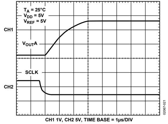
Figure 21. Half-Scale Settling (1/4 to 3/4 Scale Code Change)
