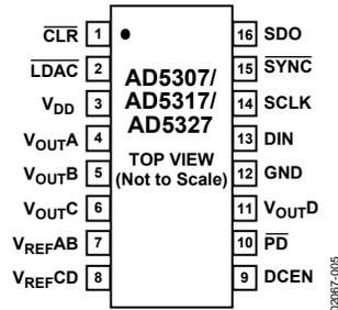
Figure 5. Pin Configuration
