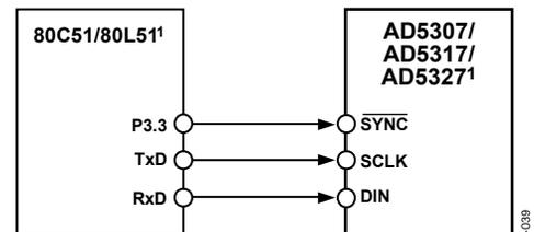
Figure 39. 80C51/80L51-to-AD5307/AD5317/AD5327 Interface
