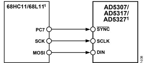
Figure 38. 68HC11/68L11-to-AD5307/AD5317/AD5327 Interface
