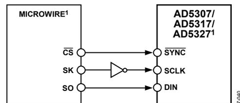
Figure 40. MICROWIRE-to-AD5307/AD5317/AD5327 Interface
