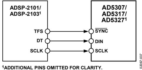
Figure 37. ADSP-2101/ADSP-2103-to-AD5307/AD5317/AD5327 Interface
