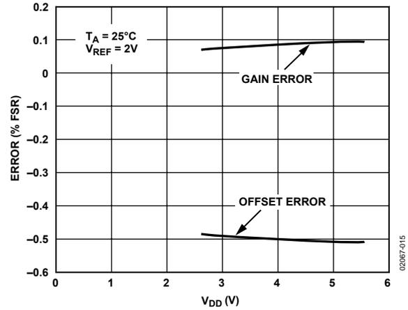
Figure 15. Offset Error and Gain Error vs.  $V_{DD}$
