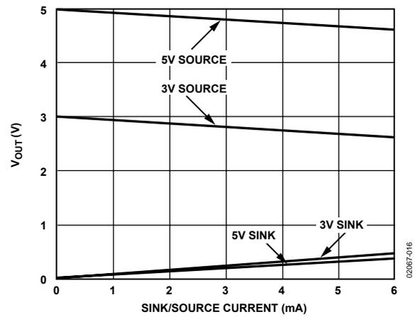
Figure 16.  $V_{out}$  Source and Sink Current Capability
