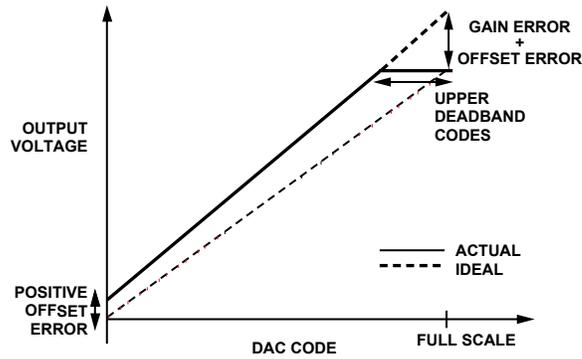
Figure 30. Transfer Function with Positive Offset ( $V_{REF} = V_{DD}$ )
