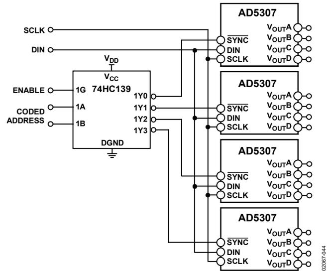
Figure 44. Decoding Multiple AD5307 Devices in a System
