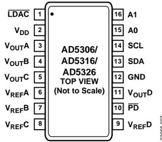
Figure 3. Pin Configuration
