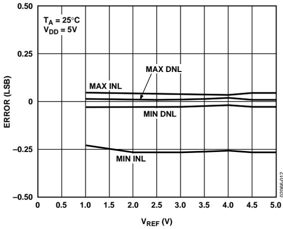
Figure 12. AD5306 INL and DNL Error vs.  $V_{REF}$
