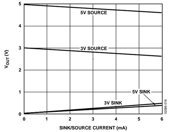
Figure 16.  $V_{OUT}$  vs. Source and Sink Current Capability
