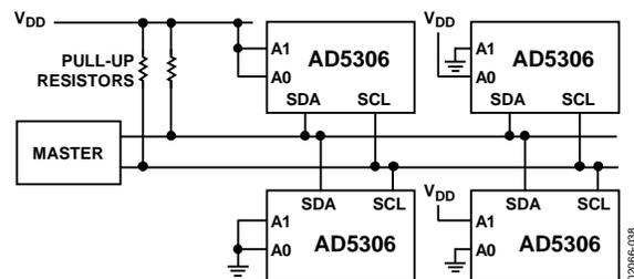
Figure 38. Multiple AD5306 Devices on One Bus
