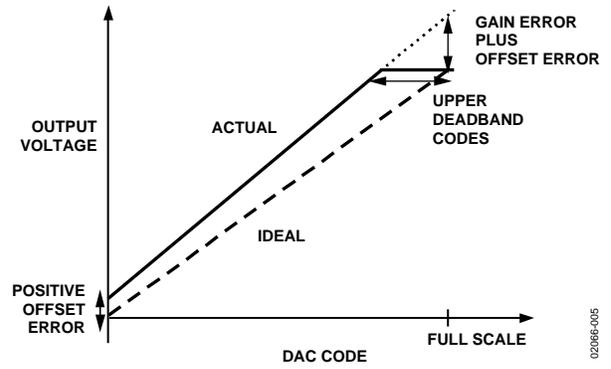
Figure 5. Transfer Function with Positive Offset ( $V_{REF} = V_{DD}$ )
