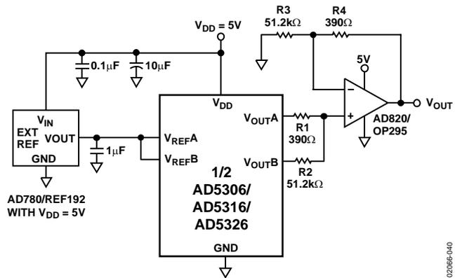
Figure 40. Coarse/Fine Adjustment
