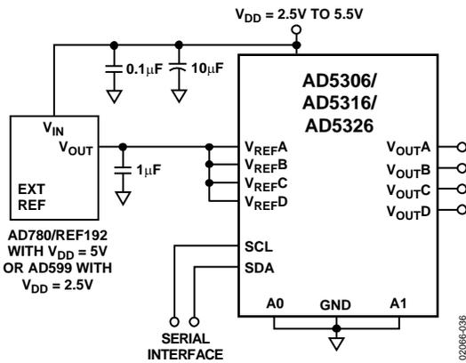
Figure 36. AD5306/AD5316/AD5326 Using a 2.5 V External Reference
