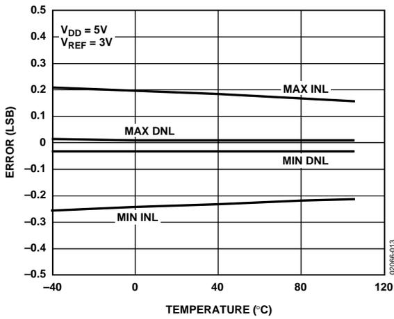
Figure 13. AD5306 INL and DNL Error vs. Temperature
