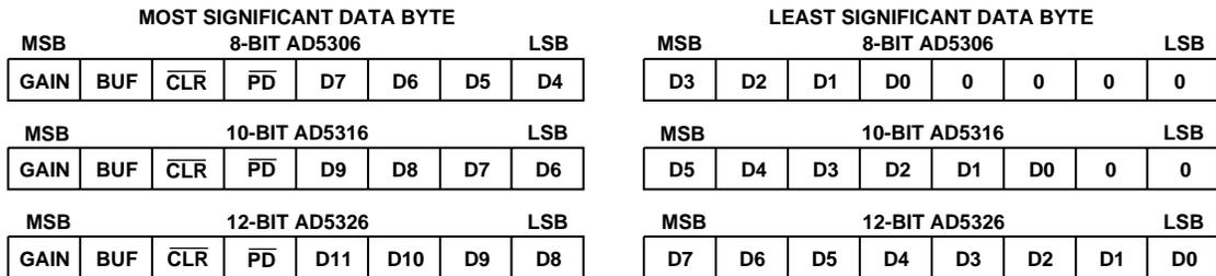
Figure 32. Data Formats for Write and Readback
