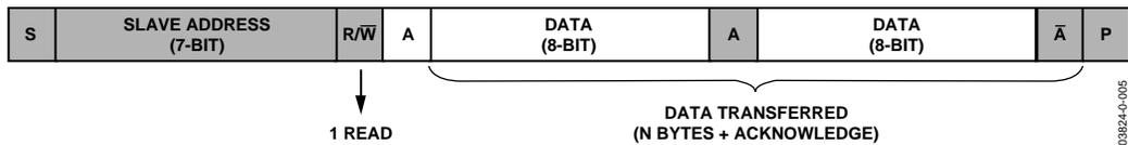
Figure 25. I<sup>2</sup>C—Master Reading Data from Slave
