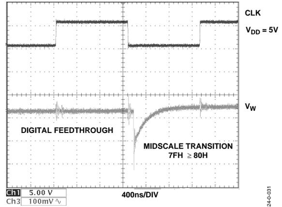
Figure 19. Clock Feedthrough and Midscale Transition Glitch
