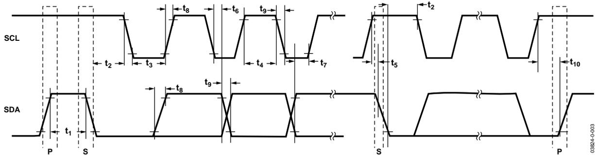
Figure 23. I<sup>2</sup>C Interface Timing Diagram
