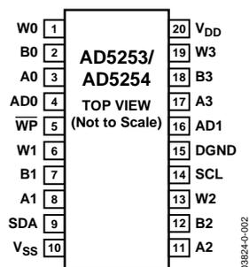
Figure 2. Pin Configuration
