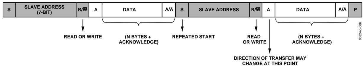
Figure 26. I<sup>2</sup>C—Combined Write/Read
