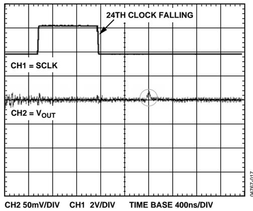
Figure 23. AD5060 Digital-to-Analog Glitch Impulse (See Figure 24)
