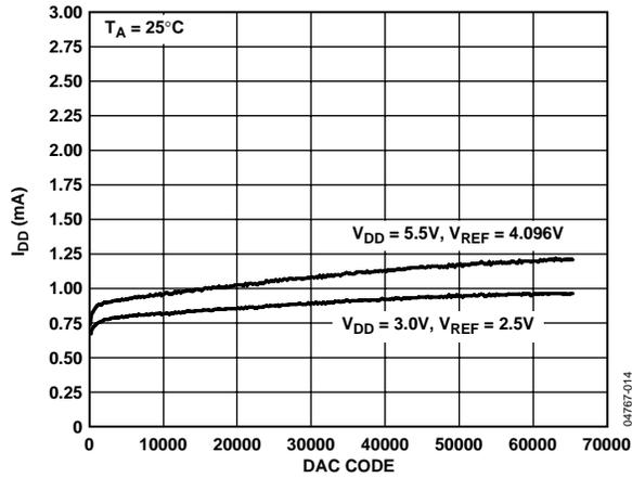
Figure 22. Typical Supply Current vs. Digital Input Code<sup>1</sup>
