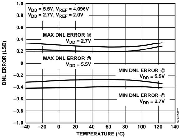
Figure 16. Typical DNL Error vs. Temperature<sup>1</sup>
