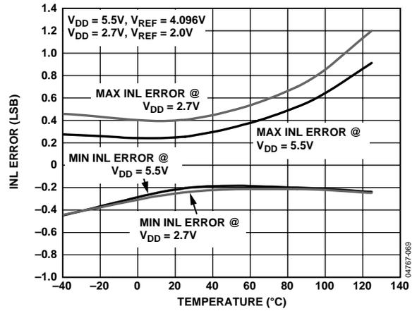
Figure 15. Typical INL Error vs. Temperature<sup>1</sup>
