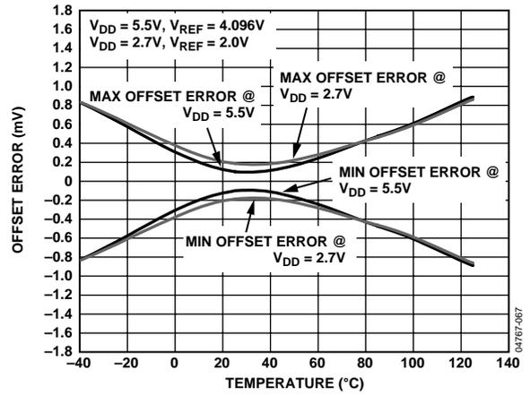
Figure 13. Typical Offset Error vs. Temperature<sup>1</sup>
