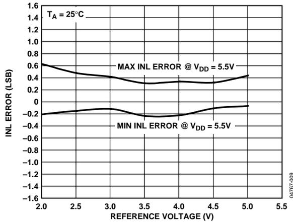
Figure 10. INL vs. Reference Input Voltage<sup>1</sup>
