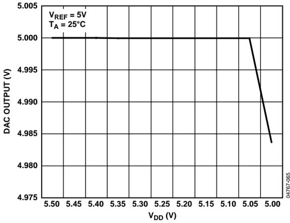
Figure 28. Typical Output vs. Supply Voltage
