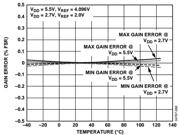
Figure 14. Typical Gain Error vs. Temperature<sup>1</sup>
