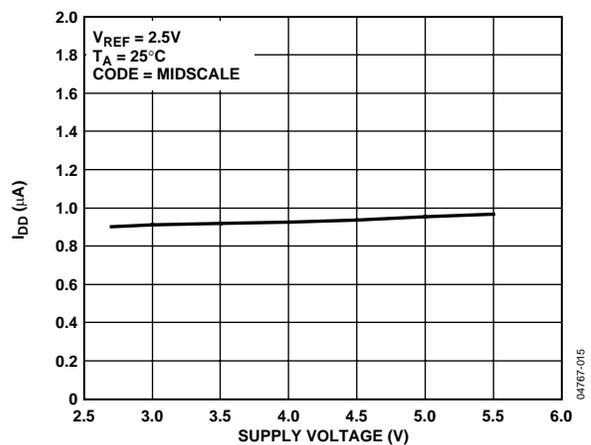
Figure 21. Typical Supply Current vs. Supply Voltage<sup>1</sup>
