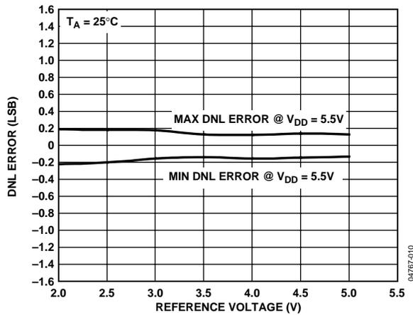
Figure 11. DNL vs. Reference Input Voltage<sup>1</sup>
