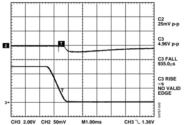
Figure 33. Glitch upon Entering Hardware Power-Down to Three-State
