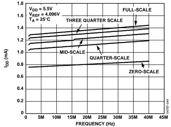
Figure 19. Typical Supply Current vs. Frequency @ 5.5 V<sup>1</sup>
