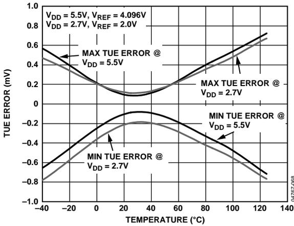
Figure 17. Typical TUE Error vs. Temperature<sup>1</sup>
