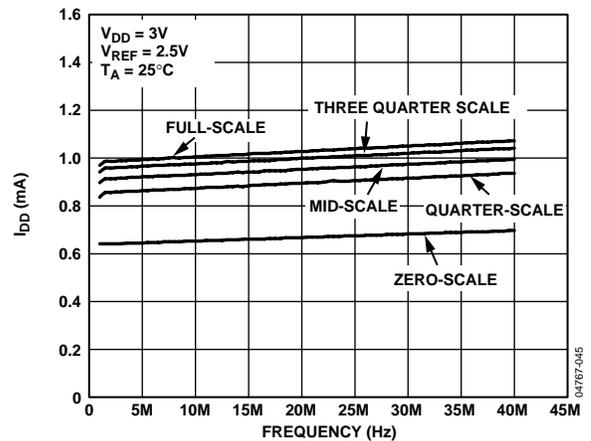
Figure 20. Typical Supply Current vs. Frequency @ 3 V<sup>1</sup>
