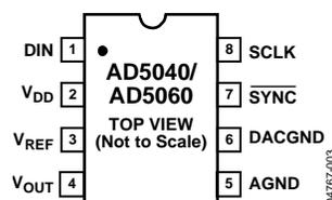
Figure 3. Pin Configuration
