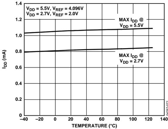
Figure 18. Typical Supply Current vs. Temperature<sup>1</sup>
