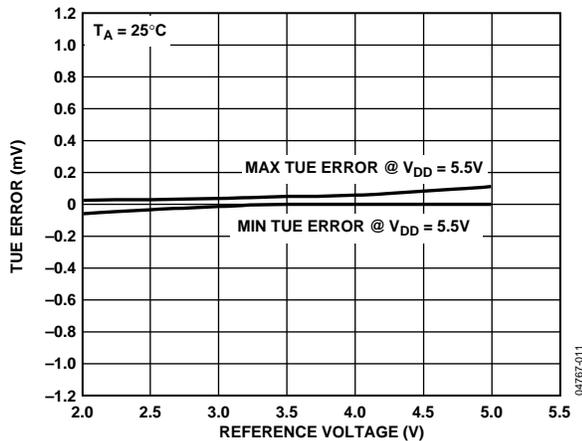
Figure 12. TUE vs. Reference Input Voltage<sup>1</sup>
