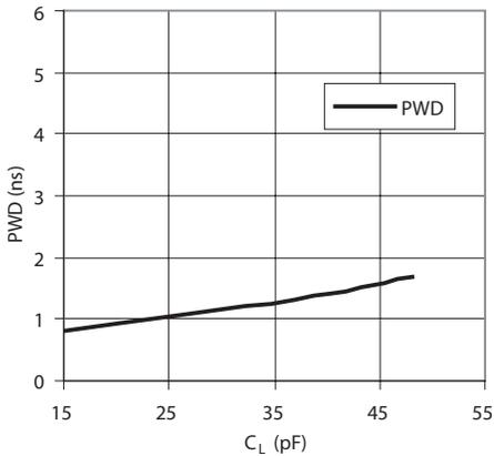
Figure 5. Typical pulse width distortion vs load capacitance
