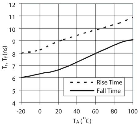
Figure 3. Typical rise and fall time vs temperature
