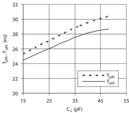
Figure 4. Typical propagation delays vs load capacitance
