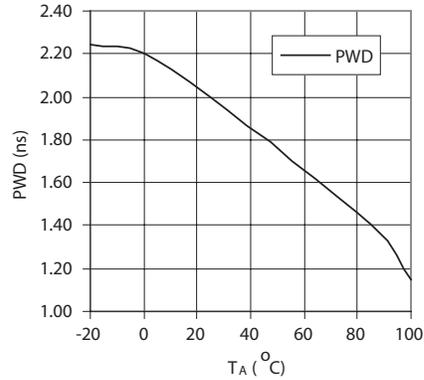
Figure 2. Typical pulse width distortion vs temperature
