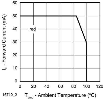
Figure 1. Max. Permissible Forward Current vs. Ambient Temperature
