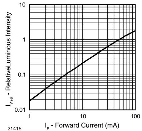
Figure 5. Relative Luminous Intensity vs. Forward Current
