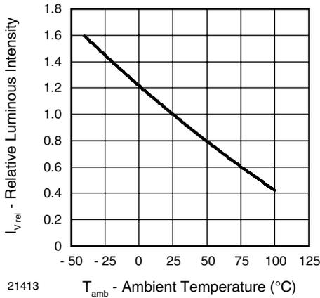
Figure 8. Relative Luminous Intensity vs. Ambient Temperature
