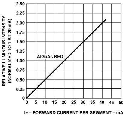
Figure 4. Relative luminous intensity vs. DC forward current.
