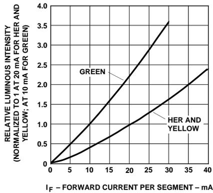
Figure 10. Relative luminous intensity vs. DC forward current.
