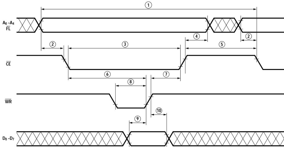
INPUT PULSE LEVELS: 0.6 V to 2.4 V
