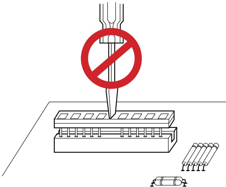
Figure 9. Improper method to manually insert a display.
