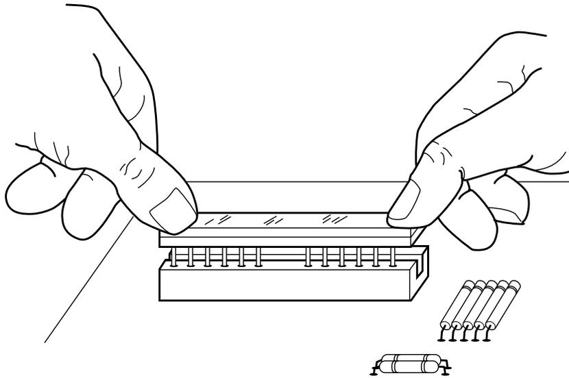
Figure 8. Proper method to manually insert a display.
