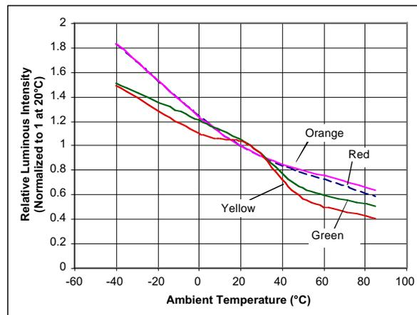
Figure 10. Relative luminous Intensity versus ambient temperature.
