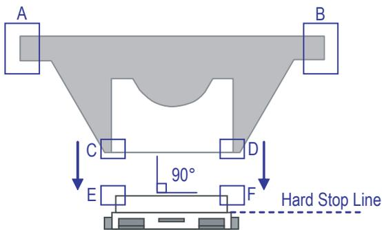
Figure 2. Attachment between collimator lens and unit.
