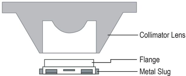
Figure 1. Collimator Lens ASMT-M0xx and ASMT-Mxxx unit
