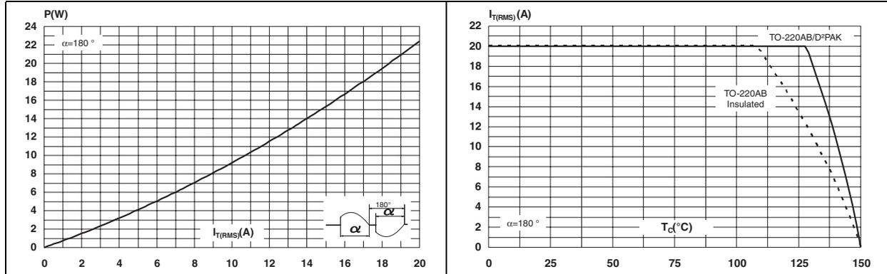
**Figure 3. On-state rms current versus ambient temperature**
