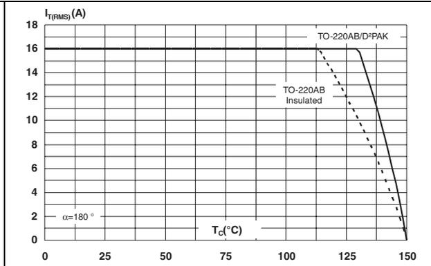
**Figure 3. RMS on-state current versus ambient temperature (Epoxy printed circuit board FR4, copper thickness = 35 μm)**
