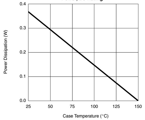
\*The power dissipation  $P_D$  is based on  $T_{J(max)} = 150^\circ\text{C}$ , using junction-to-case thermal resistance, and is more useful in settling the upper dissipation limit for cases where additional heatsinking is used. It is used to determine the current rating, when this rating falls below the package limit.
