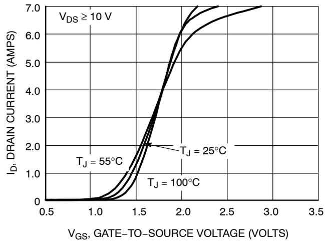
**Figure 2. Transfer Characteristics**
